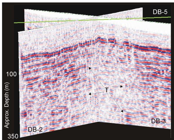
**Figure 5:** Fence diagram of the intersecting seismic profiles DB-2 and DB-3. Truncations marking the extremities of the ring-fault system discussed in the text (and plotted in plan view in Figure 2) are indicated by the label 'T'. The view is looking toward the north. The surface location of profile DB-5 (Figure 4) is indicated by the green line.
