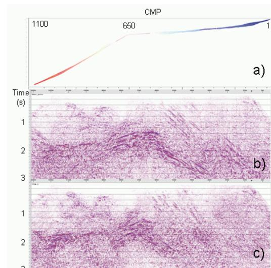
**Figure 13:** a) Seismic line track recorded over prospective gold deposits, b) DMO stack and c) post stack time migration. Note that shallow steeply dipping events migrate in expected positions. Deeper reflections are stronger and more coherent in b) than in c).
