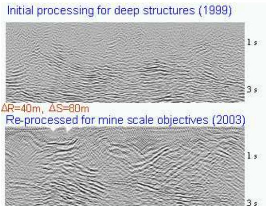
Figure 2: Initial (top) and Curtin re-processed 1999 seismic regional line (bottom).
