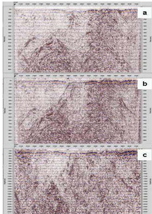
**Figure 10:** A high-resolution seismic line: a) simple stack, b) DMO-stack and c) migrated DMO stack. Note enhanced steeply dipping events after application of DMO corrections.
