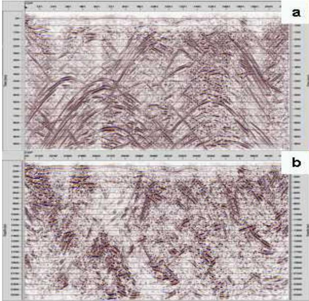
**Figure 11:** a) Multifocussing stack (Courtesy of Geomage.) and b) migrated multifocussing stack. Compare these two images to the equivalent DMO and DMO migrated stacks of Figure 10.
