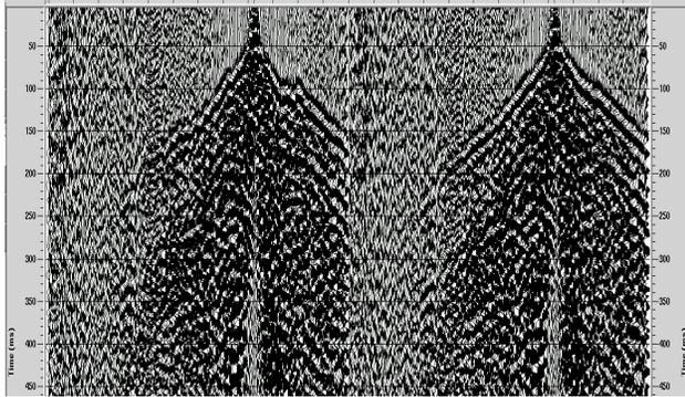
**Figure 6:** Stack with refraction statics applied (upper image) and stack with refraction and residual refraction statics applied (lower image).
