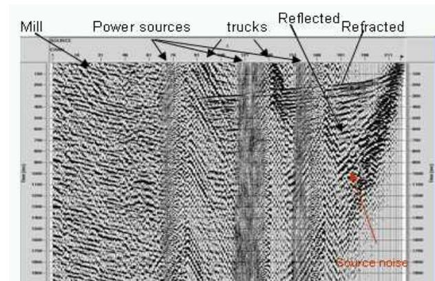
Figure 4: Shot recorded during active mine operations. Various noise sources are labelled.
