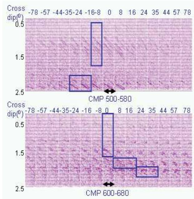
**Figure 14:** Crossdip analysis. Shallow reflections display small crossline dip angle. Dipper structural shapes appear more complex (lower panel, CMP range 600-680).
