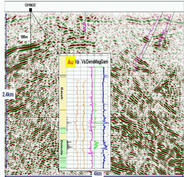
**Figure 18:** Direct targeting of gold bearing structures from seismic data. Two boreholes (pink impedance logs) struck gold bearing ore bodies at 600 m and 1000 m, respectively within 10m of predicted depth.
