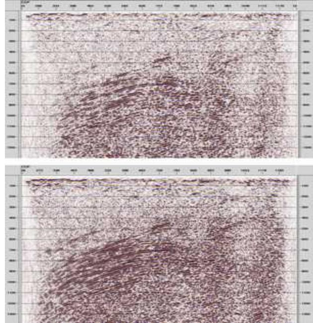
**Figure 7:** Stacks with refraction statics applied (upper) and residual refraction statics applied (lower).
