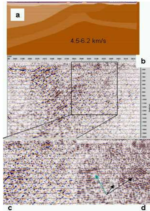
**Figure 12:** a) Velocity model in depth, b) Depth migrated DMO stack, c) enlarged part of image in B) and d) equivalent PSDM image (Kirchhoff integral method). Clearly the imaging results can be distinctly different and a priori knowledge of geology is helpful in estimating an optimum output.
