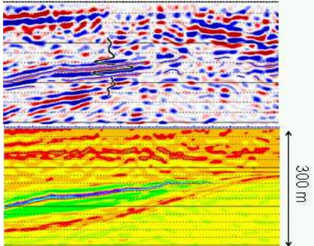
**Figure 20:** Model-based impedance inversion used for targeting gold bearing dolerites.
