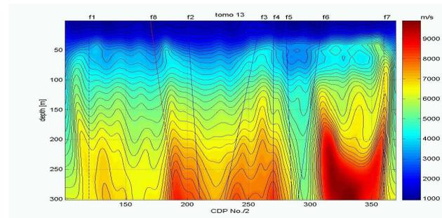
**Figure 8:** Refraction tomography used to delineate near surface (regolith) discontinuities. Faults overlaid are from drilling information.
