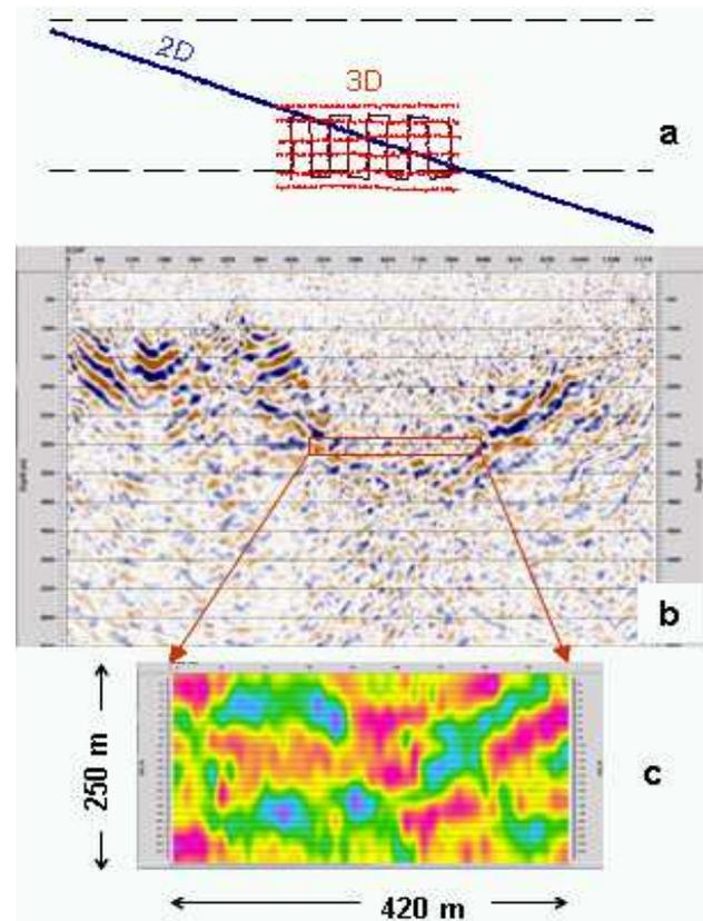
**Figure 16:** Experimental seismic survey: a) 2D and 3D surface layout. Receiver lines shown in blue, shot lines in red. b) 2D migrated stack and c) Time slice from 3D mini data cube.
