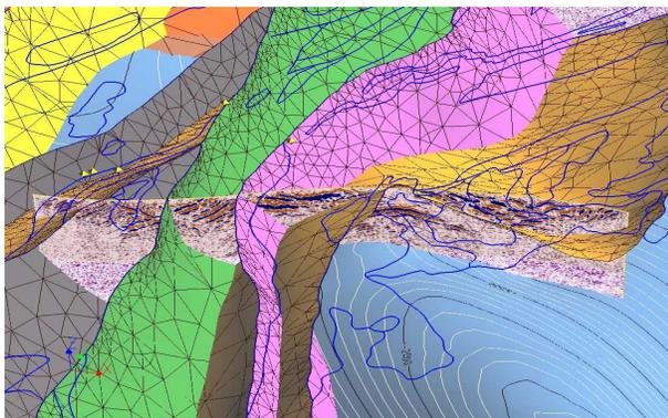
Figure 3: Reprocessed seismic image verified against known geology.
