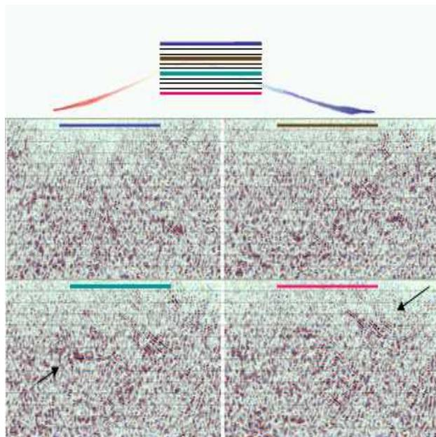
**Figure 15:** 3D PSDM of a crooked line segment. Position of the output in-line and the corresponding image are colour connected. Note that last two images (green and blue) which are far away from the central track show most coherent images.
