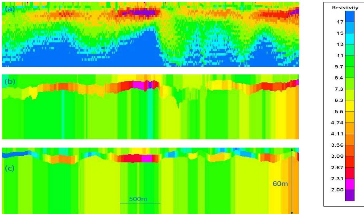
**Figure 2:** Inversion results from the survey data in Texas Levees area. (a) CDT section; (b) 3-layer SVD inversion; (c) 3-layer SA inversion. The resistivity unit is ohm-m. Data courtesy of U.S. Army Corps of Engineers.
