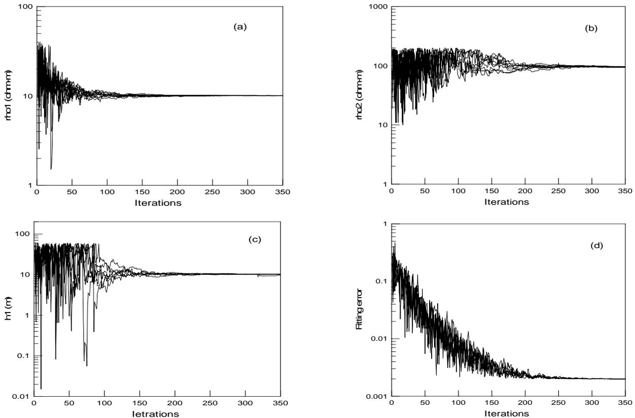
**Figure 1:** Inversion results by simulated annealing for a theoretical two-layer model. (a) First layer resistivity; (b) second layer resistivity; (c) first layer thickness; (d) fitting error.
