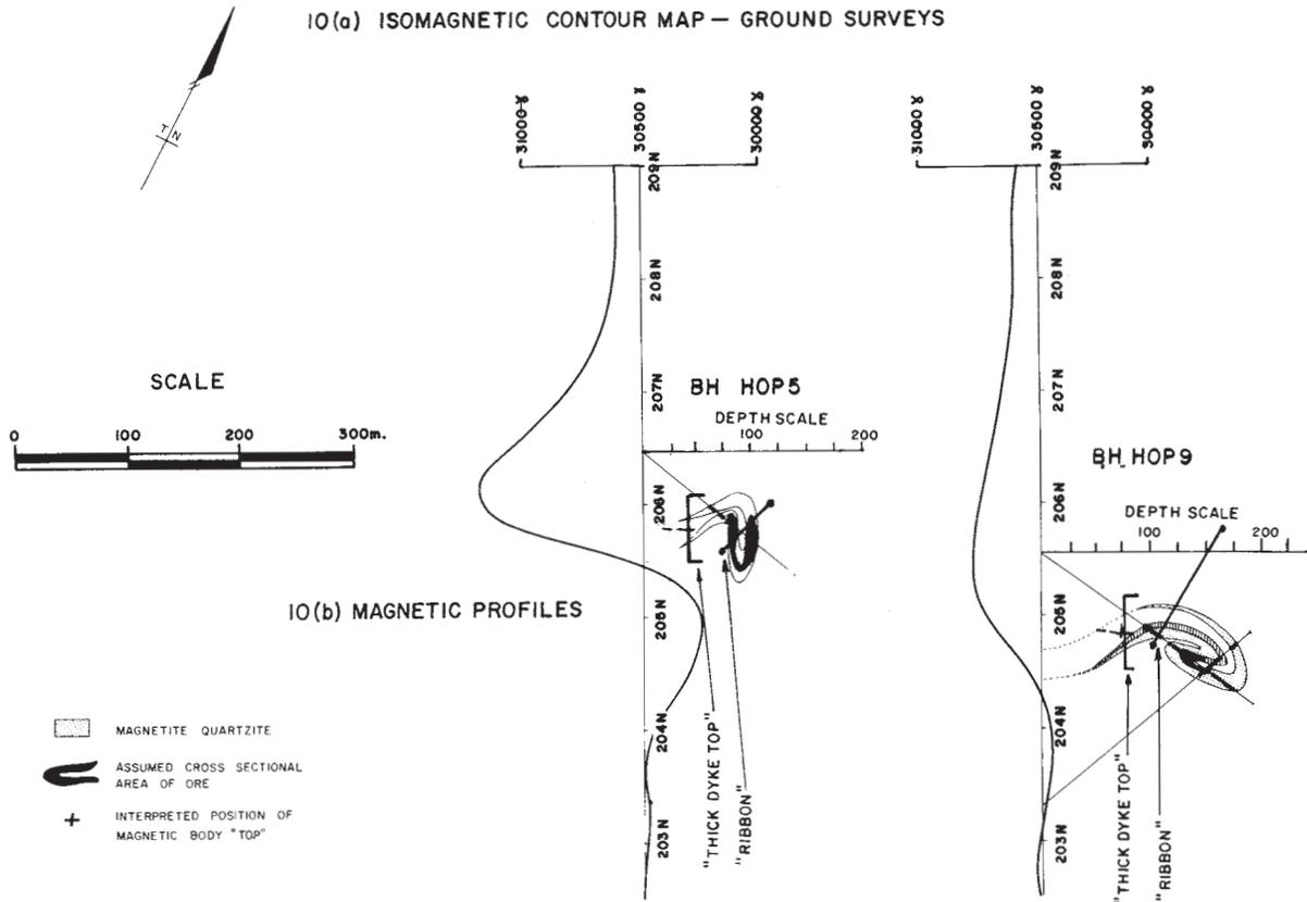
Figure 38.10. Ground magnetometer surveys, Hope Mine Zone.
