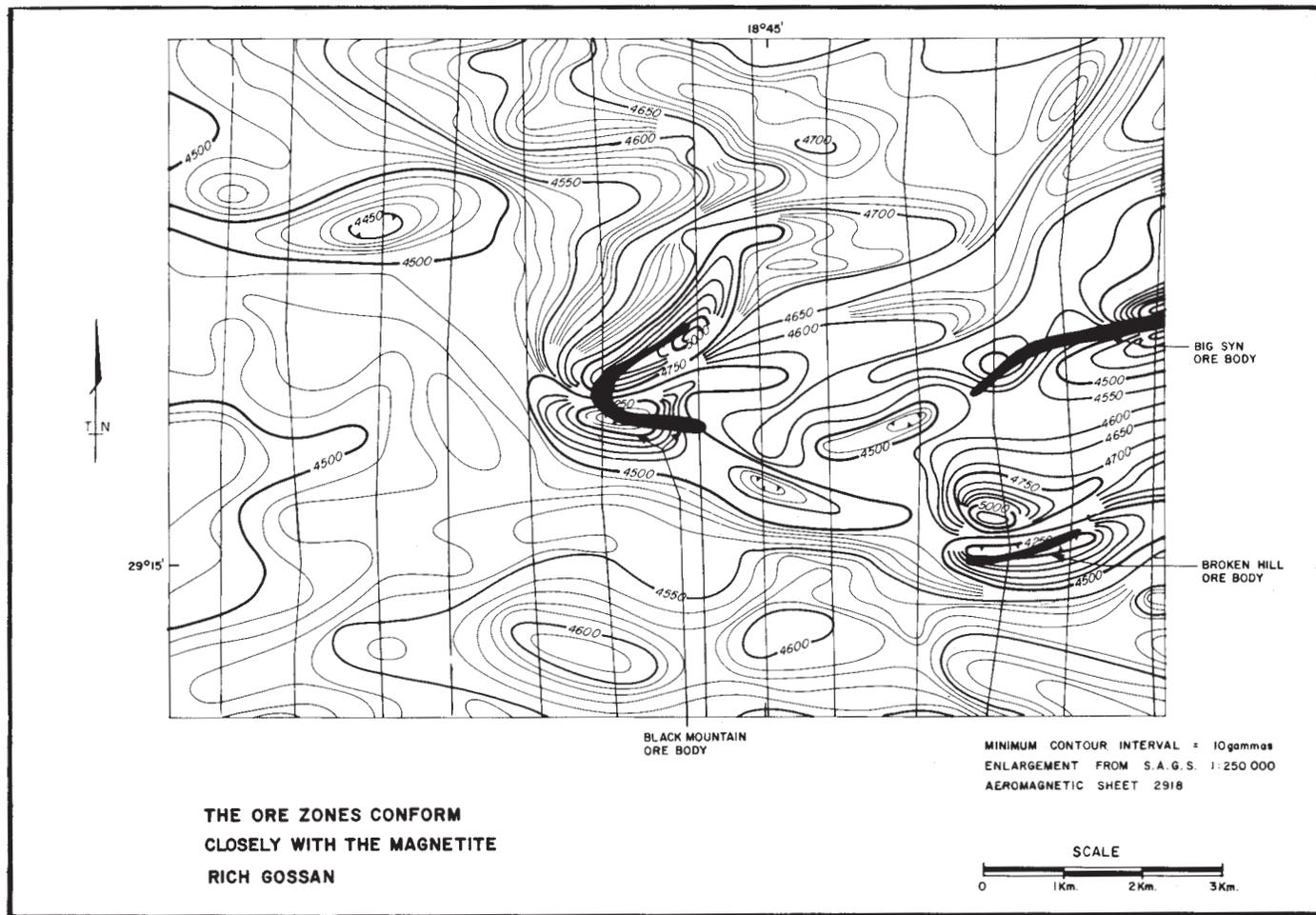
Figure 38.2. Aeromagnetic contour map, Aggenys area.
