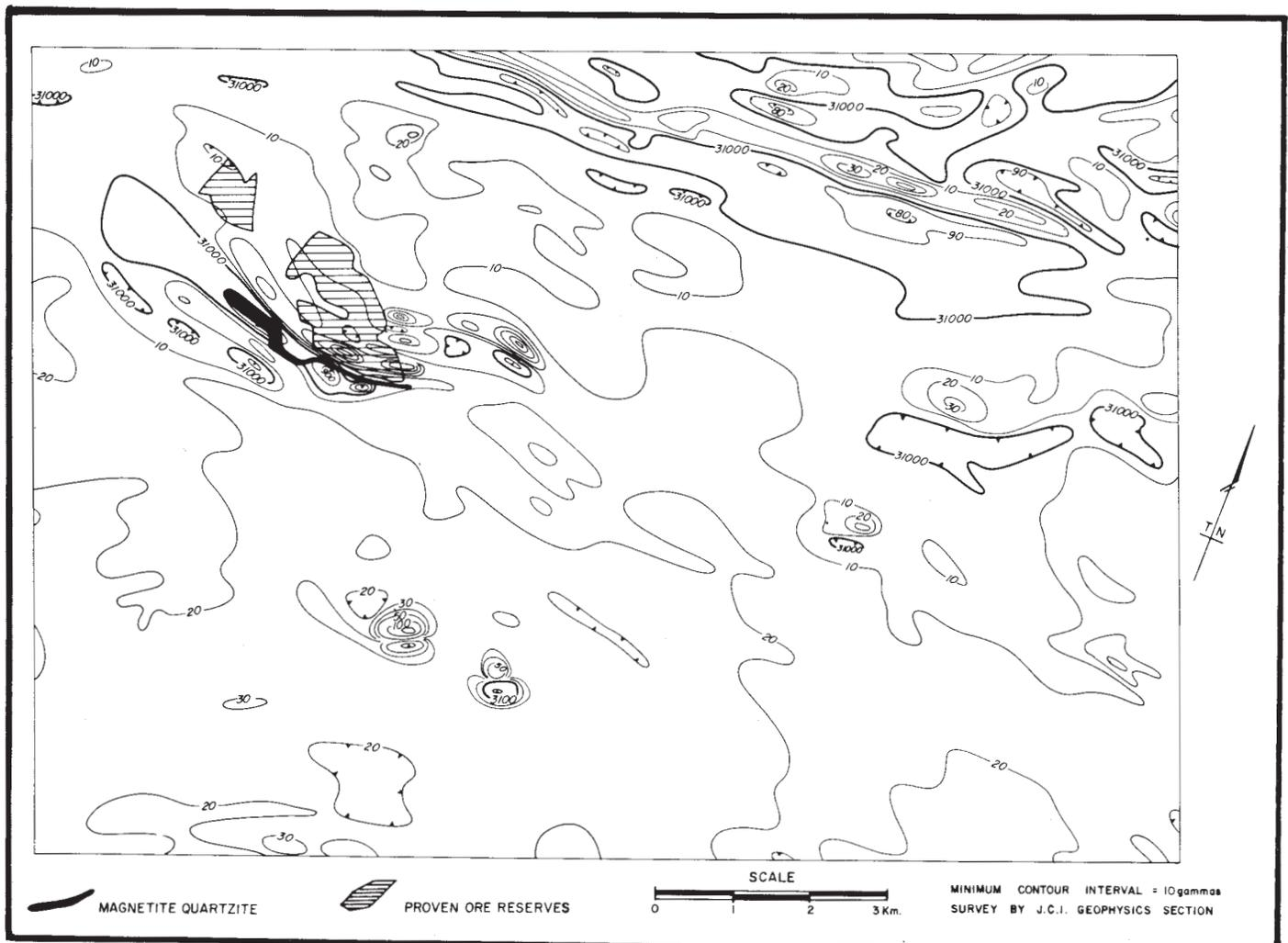
**Figure 38.3.** Aeromagnetic contour map, Otjihase area.
