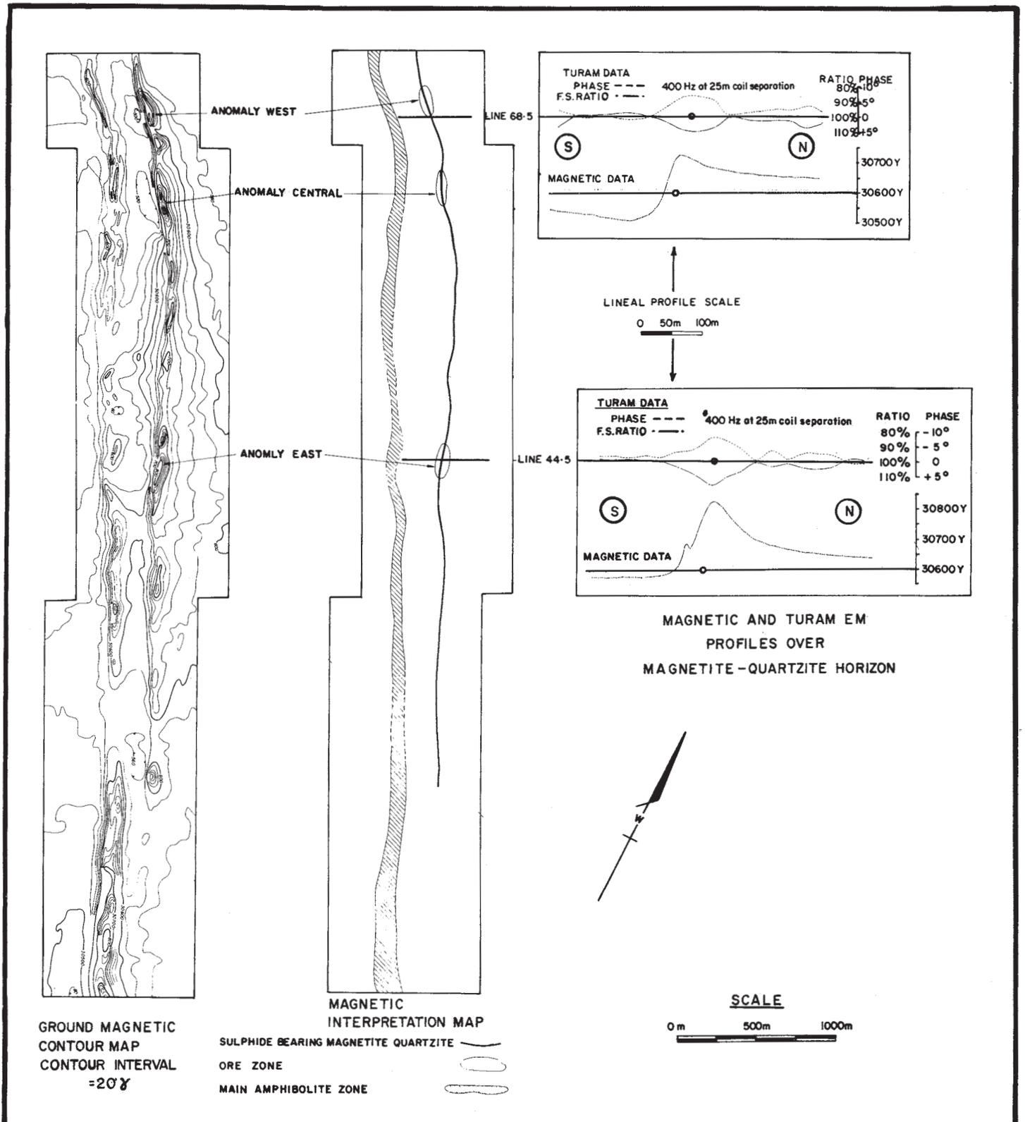
Figure 38.9. Ground geophysical surveys and interpretation, Anomaly Zone area.
