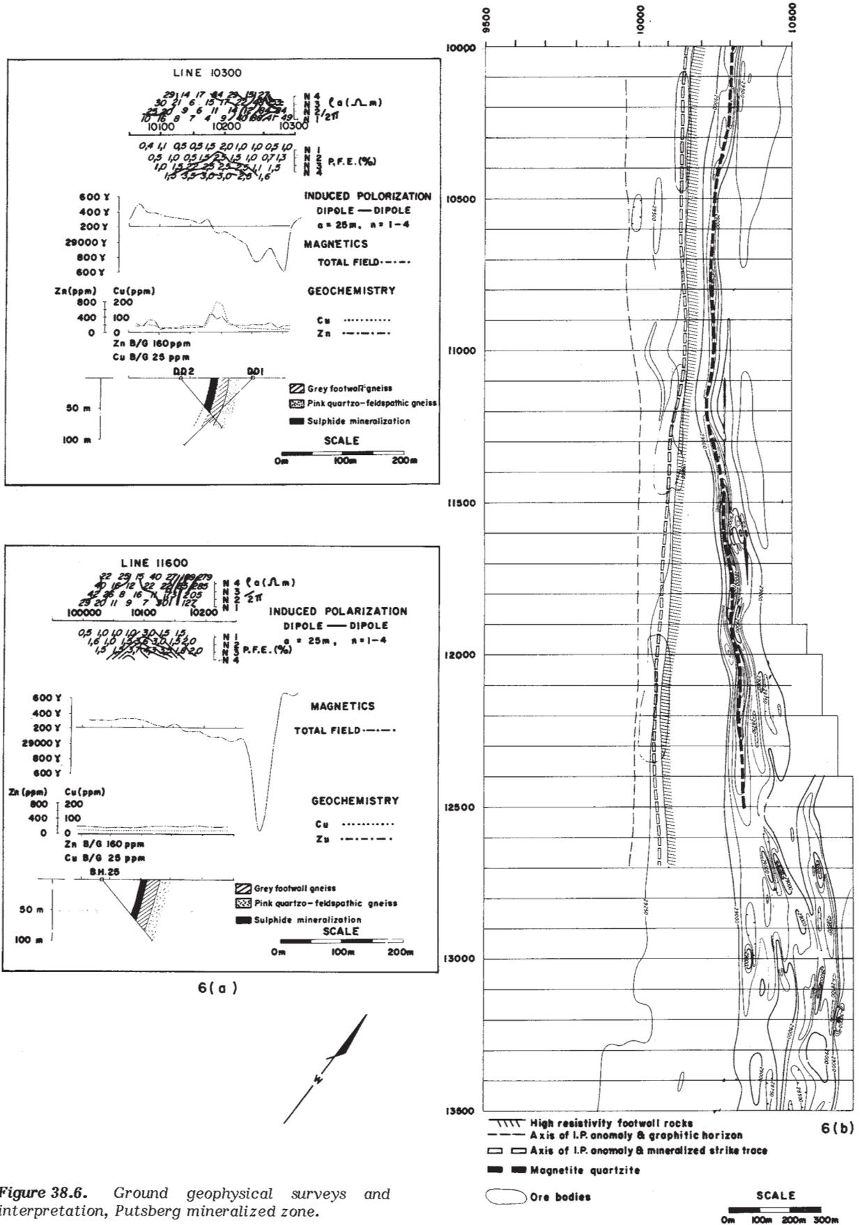
Figure 38.6. Ground geophysical surveys and interpretation, Putsberg mineralized zone.
