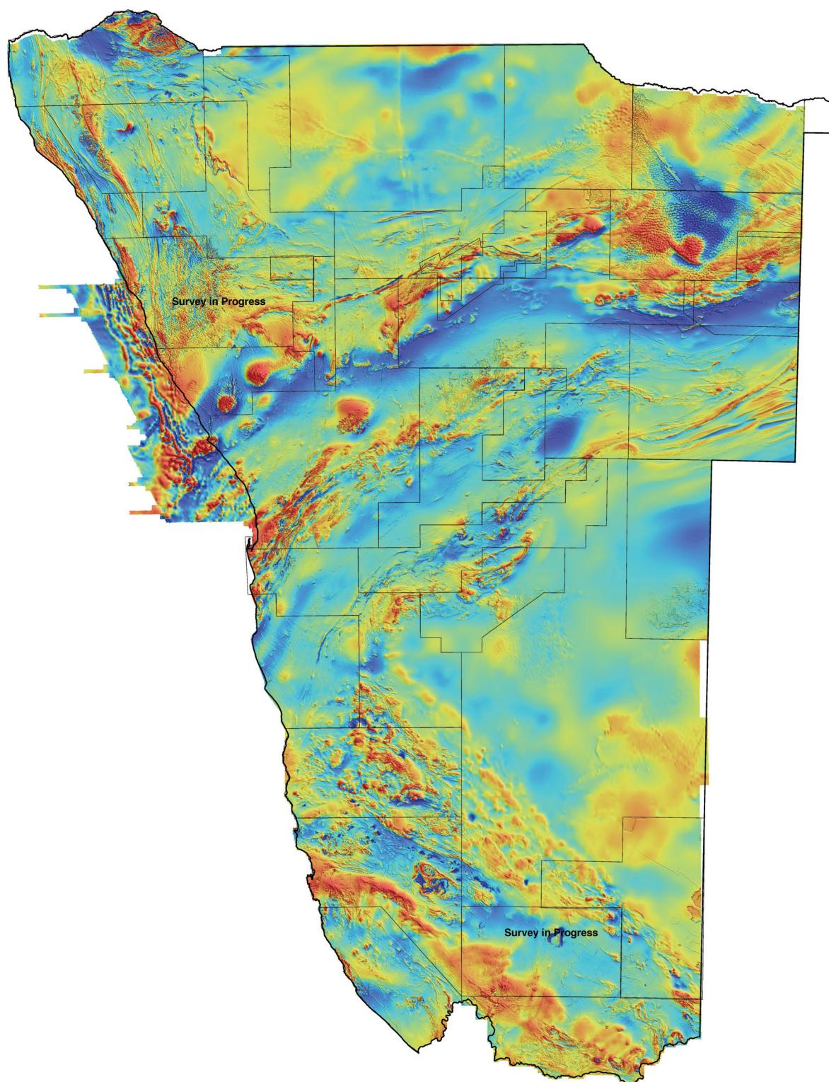
**Figure 1b:** NW shaded TMI image of the merged high-resolution and regional magnetic data of Namibia
