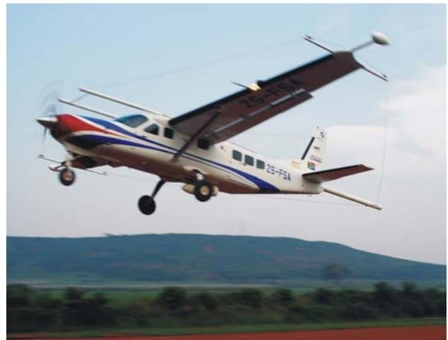
**Figure 3:** The Genesis electromagnetic system mounted on a Cessna 208B, Kakira, Uganda.
