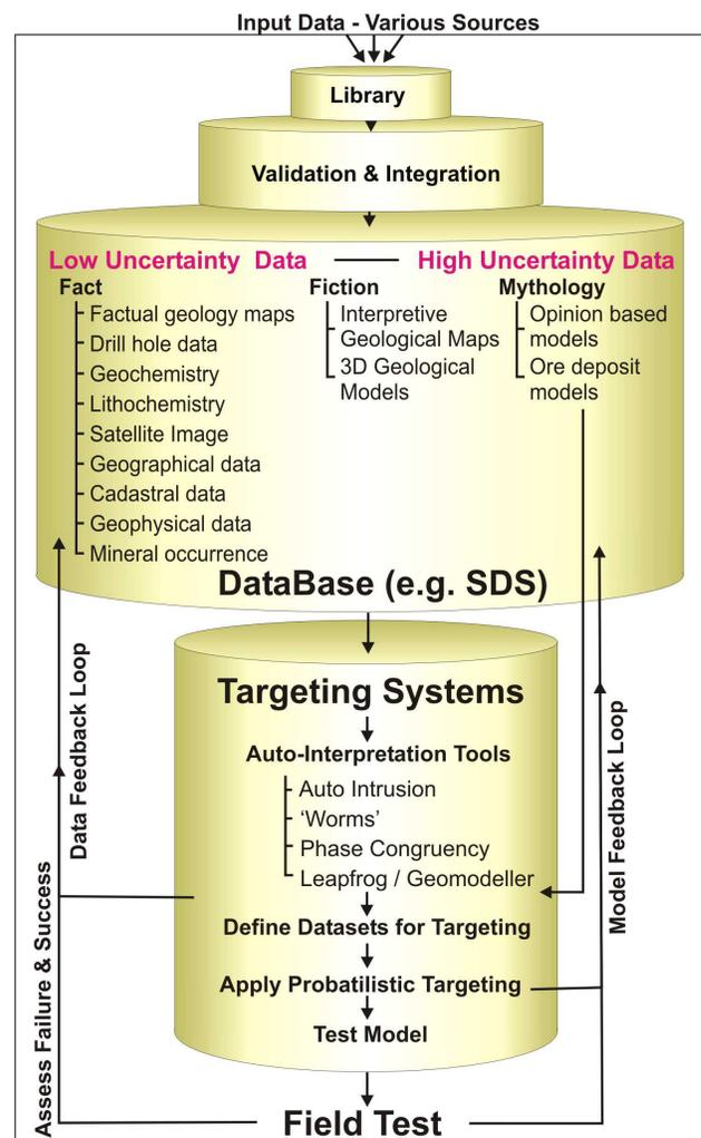
**Figure 5:** A graphical representation of Geoinformatics Data Model, and data flow; showing the separation of "Fact, Fiction & Mythology". The feedback loops allow targeting models to be better defined based on the results of the targeting process and field checking.
