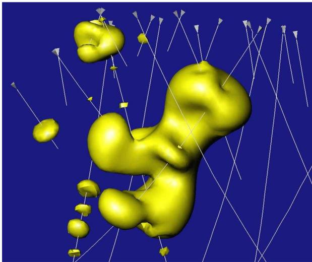
**Figure 4:** An oblique view of an automated grade-shell model created by Leapfrog software. The yellow surface represents ore at a specific cut-off grade. The white lines are drill-holes. The model is approximately 600m by 300m and modelled to a depth of 500m.
