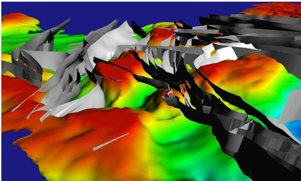
**Figure 3:** Tasmania 3D geological model, an example of a Terrane scale model constructed by Fractal Graphics. The figure shows an oblique view of the Devonian granitoids of NW Tasmania (coloured surface, intersected by major faults (grey surfaces)). The model is based on interpretations of magnetics, gravity and seismic data as well as surface interpretive geological maps. The view is approximately 300km by 200km and to a depth of 15km.
