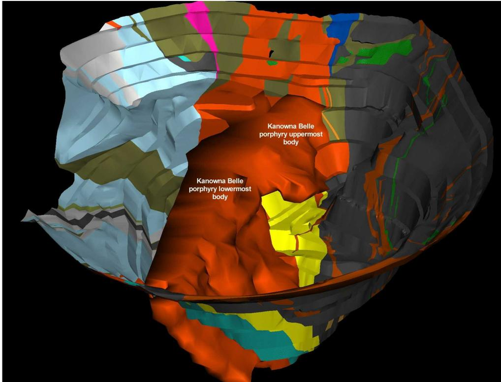
**Figure 2:** Kanowna-Belle, Western Australia - an example of in-mine geological modelling from 1997 constructed by Fractal Graphics for Delta Gold NL. The figure shows an oblique view of geological mapping draped on an open-pit shell, with a 3D model of a porphyry body within the pit. The model is based on geological mapping and drill-hole logging. The pit is approximately 800m by 600m.
