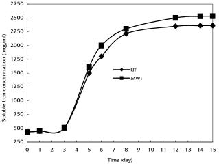
Figure 2. Change in soluble iron concentrations during biodesulphurization of microwave treated (MWT) and untreated (UT) coal
