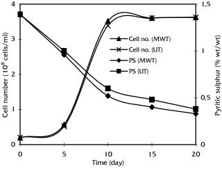
Figure 1. Change in pyritic sulphur and cell number during biodesulphurization of microwave treated (MWT) and untreated (UT) coal
