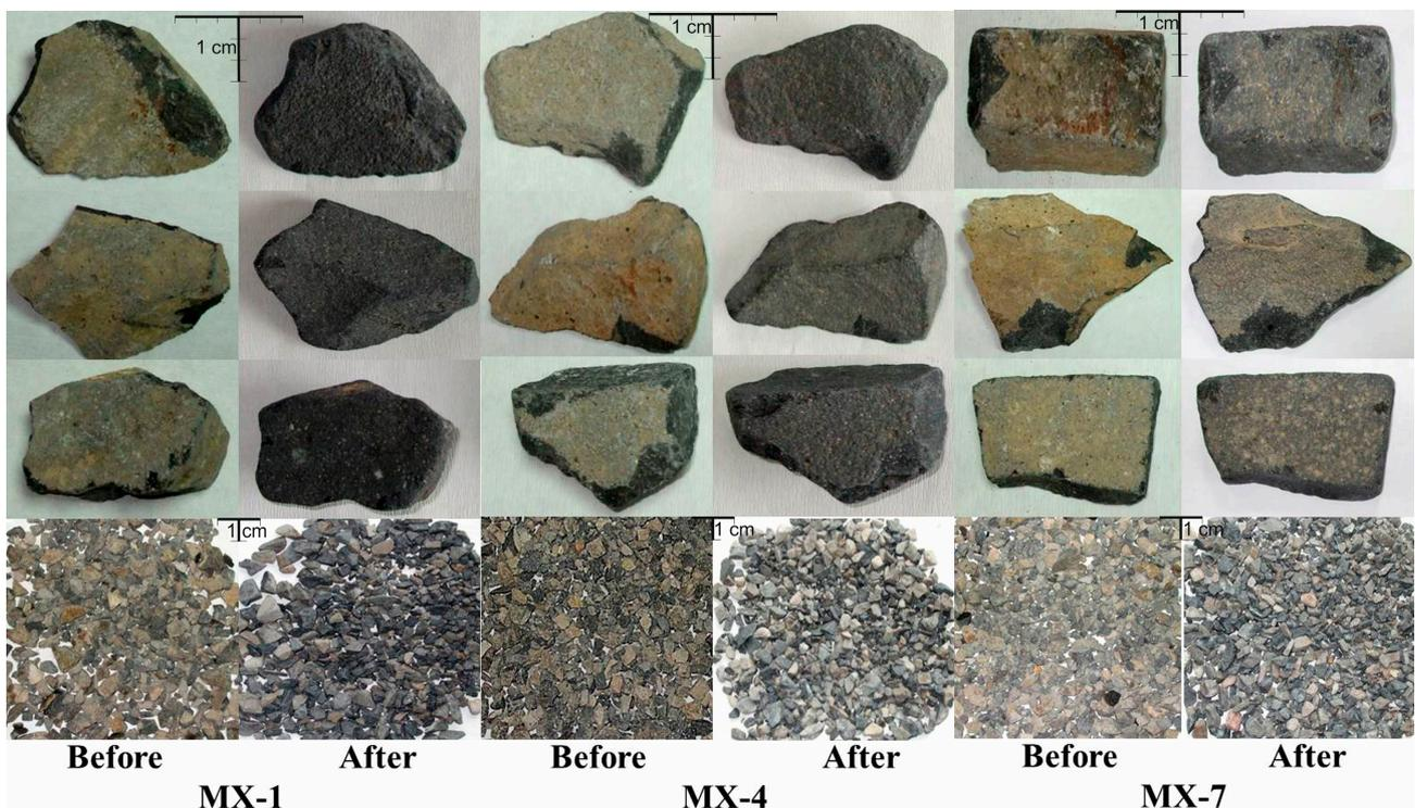
**Figure 4.** Particles of basaltic waste-rock before and after tumbling for MX-1, MX-4 and MX-7 mixtures (particles of +63 mm coarse and −22 +12 mm medium size fractions).
