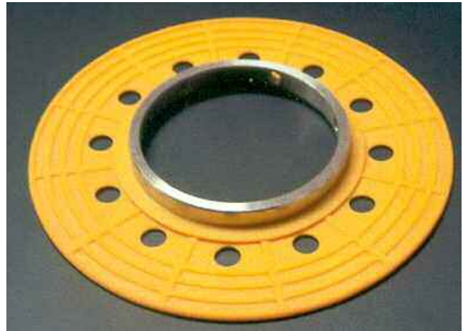
Figure 4. “Trimmable” Flinger Disc—A superior replacement for oil rings in equipment furnished with rolling element bearings. (Courtesy Trico Mfg. Co.)
