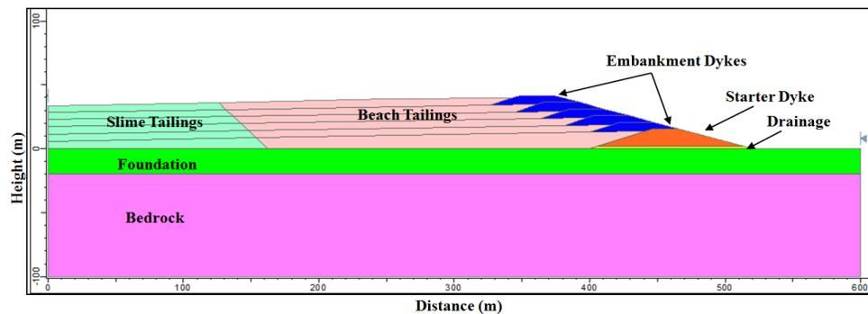
Figure 1 – Numerical model: UTSF: End of construction
