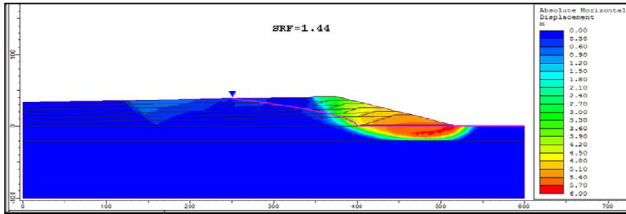
(c) Horizontal displacements using SRT
