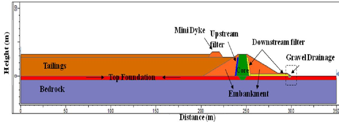
Figure 2 – Numerical model: WRTD - End of construction
