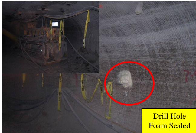
Figure 1 – Virgin rock temperature experimental station and drilling equipment (in inset)
