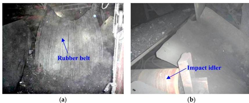
Figure 11. Buffer device: (a) rubber belt; (b) impact idler.
