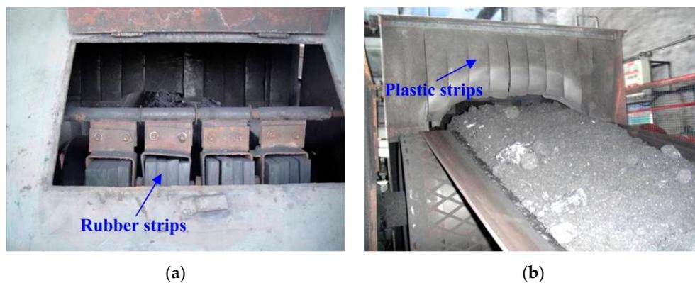
**Figure 16.** The buffer systems at transloading points: (a) rubber strips; (b) plastic strips.
