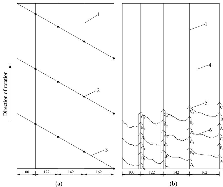
**Figure 4.** A novel shearer drum with large cutting depth and digging capabilities: (a) arrangement of cutting picks on blades; (b) cutting cross-section of kerfs; 1, transversals; 2, cutting picks; 3, blades; 4, anthracite; 5, kerfs; 6, cracks.
