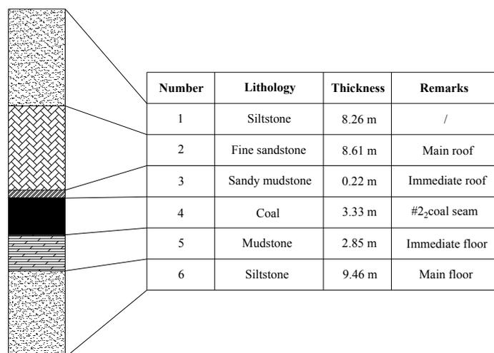
Figure 2. The generalized column of the NSP.
