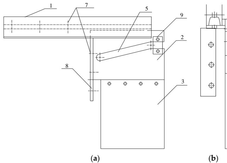
Figure 8. Schematic illustration of a side protecting plate: (a) front view; (b) side view.
