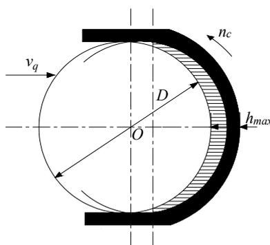
Figure 3. The ranges of drum cutting thickness.
