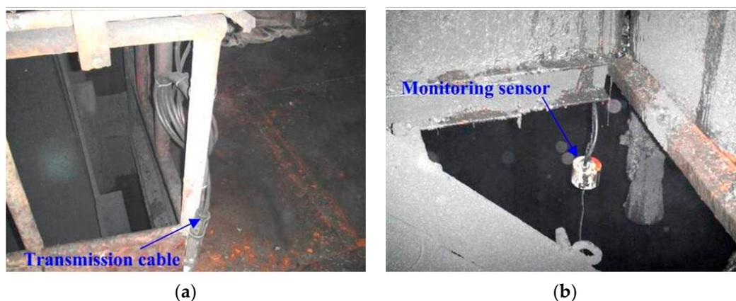
**Figure 12.** Bunker stock level monitoring system: (a) bunker opening; (b) sensor layout.
