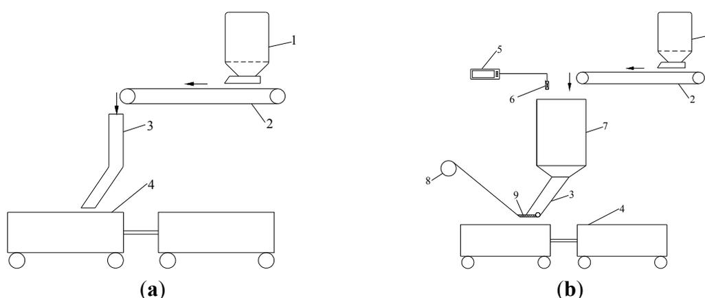
**Figure 18.** Railway wagon loading processes: (a) conventional loading system; (b) fragmentation-prevention loading system; 1, feeder; 2, belt conveyor; 3, chute; 4, railway wagon; 5, display of stock level; 6, sensor of stock level; 7, storage hopper; 8, winch; 9, valve.
