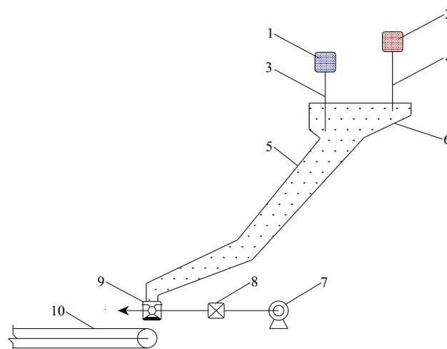
**Figure 17.** LKK-1 fragmentation-prevention system: 1, signal relay of low stock level; 2, signal relay of high stock level; 3, electrode of low stock level; 4, electrode of high stock level; 5, coal chute; 6, surge bunker; 7, electromotor; 8, gearbox; 9, impeller coal feeder; 10, main conveyor.
