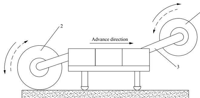
**Figure 5.** Clockwise/anti-clockwise or anti-clockwise/clockwise patterns of front and rear drums: 1, front drum; 2, rear drum; 3, rocker arm.
