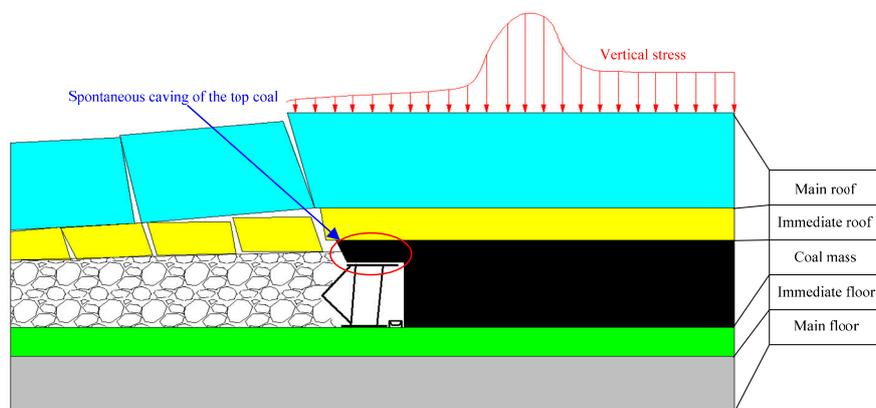
Figure 6. Schematic illustration of the coalface mining process.
