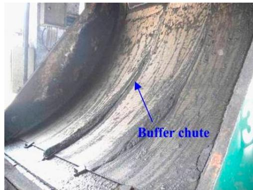
Figure 13. Buffer chute.
