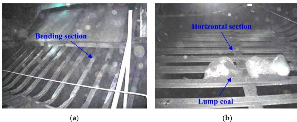
Figure 15. Interval blocking units: (a) bending section; (b) horizontal section.
