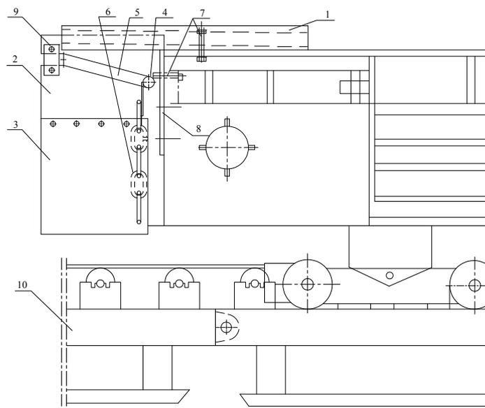
**Figure 7.** Basic configuration of the buffer unit: 1, fixed flange beam; 2, fixed side protecting plate; 3, movable side protecting plate; 4, buffer axis; 5, guide slot; 6, buffer chain; 7, fixed bolt; 8, connection plate; 9, damper; 10, extensible belt conveyor.
