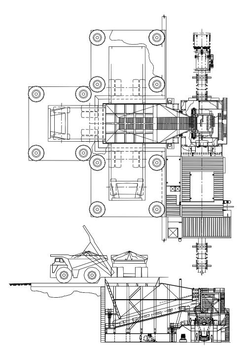
Figure 12 Typical low speed roll sizer installation
