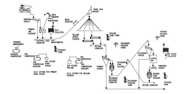
Figure 6 Three stage crushing closed circuit
