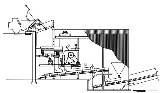
Figure 10 Typical jaw crusher plant enclosed
