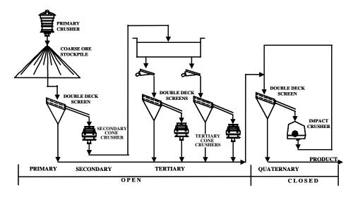
Figure 5 Four stage crushing circuit
