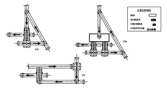
Figure 17 Typical closed circuit secondary crushing
