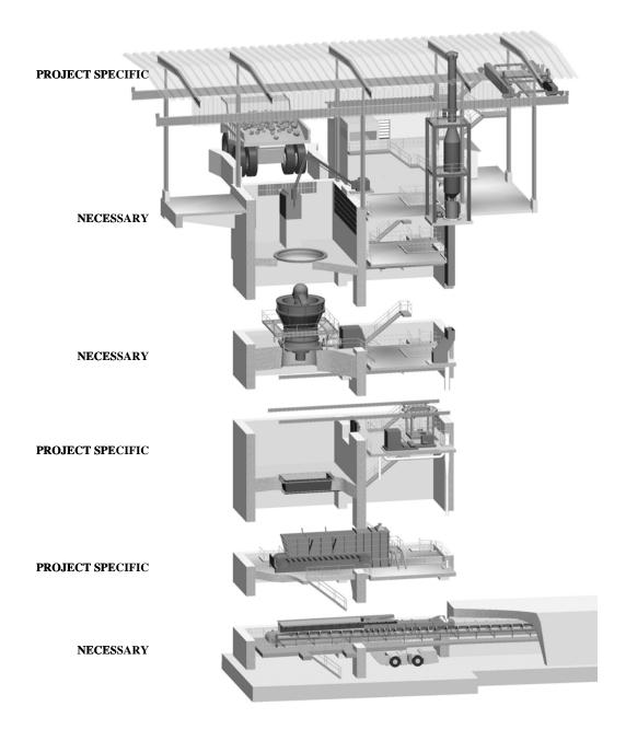
Figure 9 Gyratory broken into necessary process portions and project specific portions
