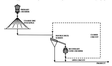
Figure 3 Two stage open/closed circuit
