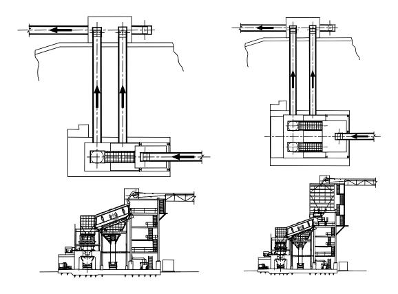
Figure 13 Open circuit (1) secondary crusher
