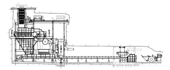
Figure 11 Typical underground jaw crusher installation
