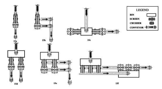
Figure 15 Typical open circuit secondary crusher options
