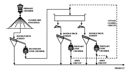
Figure 4 Three stage open/closed circuit
