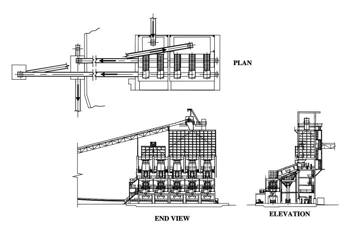
Figure 19 Typical secondary and tertiary closed circuit layout
