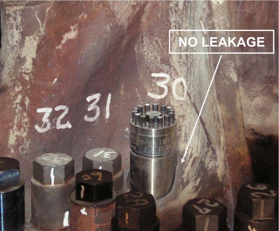
IMPROVED HORIZONTAL JOINT WITH ADVANCED STUDS AND ADVANCED TENSIONERS
