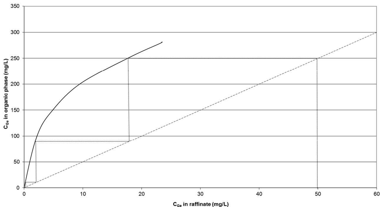
**Figure 3.** McCabe-Thiele diagram of extraction system.
