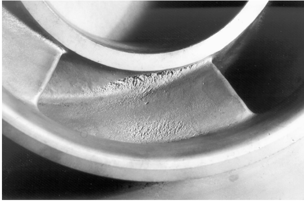
Figure 2. Cavitation Erosion on High-Energy Suction Stage Impeller. (Evidence of sheet cavitation and hub fillet cavitation as seen by the erosion patterns.)
