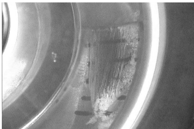
Figure 1. Typical Sheet Cavitation Pattern on High-Energy Feed Pump Impeller Blade.
