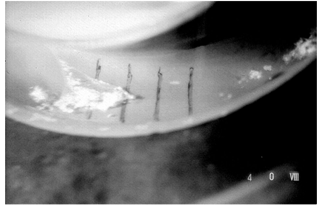
Figure 13. Cavitation Vapor on Biased-Wedge Impeller Blade Operating at 35 Percent BEP Flow Rate. (This shows the impeller is similar in performance to the impeller shown in Figure 12, and uses biased-wedge shaped blades.)
