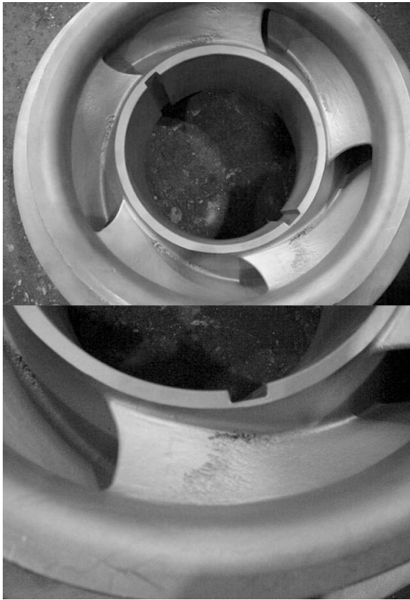
Figure 15. Improved Suction Impeller for Fossil Fuel Plant in Louisiana.
