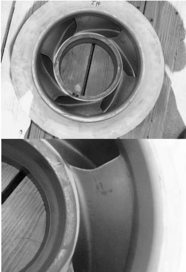
Figure 10. Improved Impeller after Four Years' Service.
