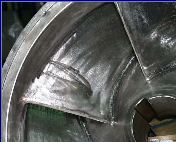
SURFACE FINISH IMPROVEMENT – UNDERFILE DETAILS
