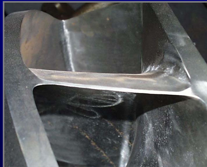
SURFACE FINISH IMPROVEMENT – UNDERFILE DETAILS
