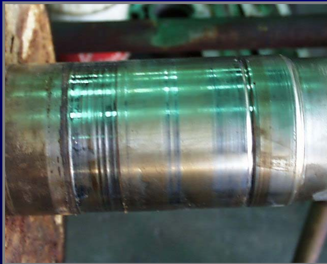
WORN SHAFT SLEEVE
