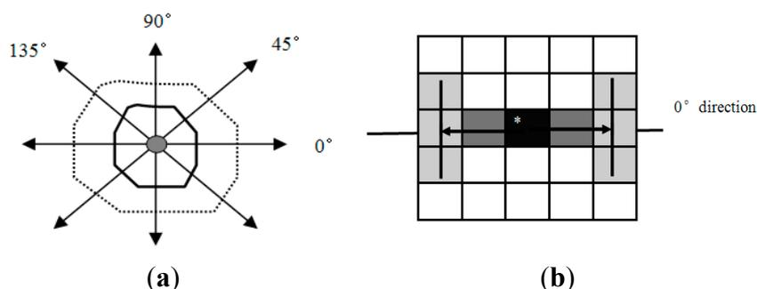
**Figure 4.** Diagram for detection algorithm. (a) The four directions; (b) detection template in  $0^\circ$  direction of a froth image of large bubbles.
