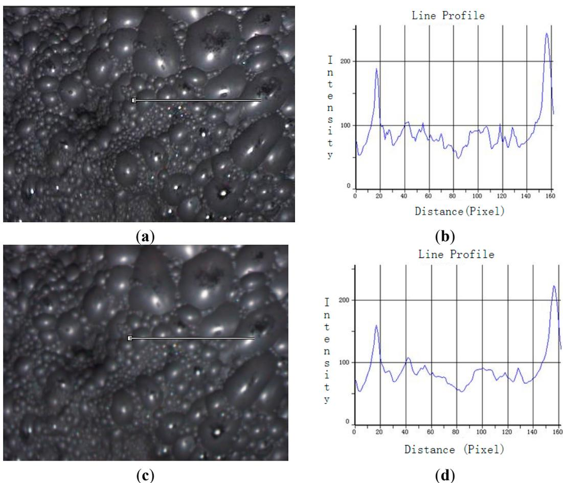
**Figure 7.** Gray value variance comparison before and after Gaussian filtering. **(a)** Original froth image and a profile line; **(b)** Gray value histogram of the profile corresponding to the image (a) from left to right; **(c)** Result smoothed by the Gaussian filter and profile line at the same position; **(d)** Gray value histogram of the profile corresponding to the image (c) from left to right.
