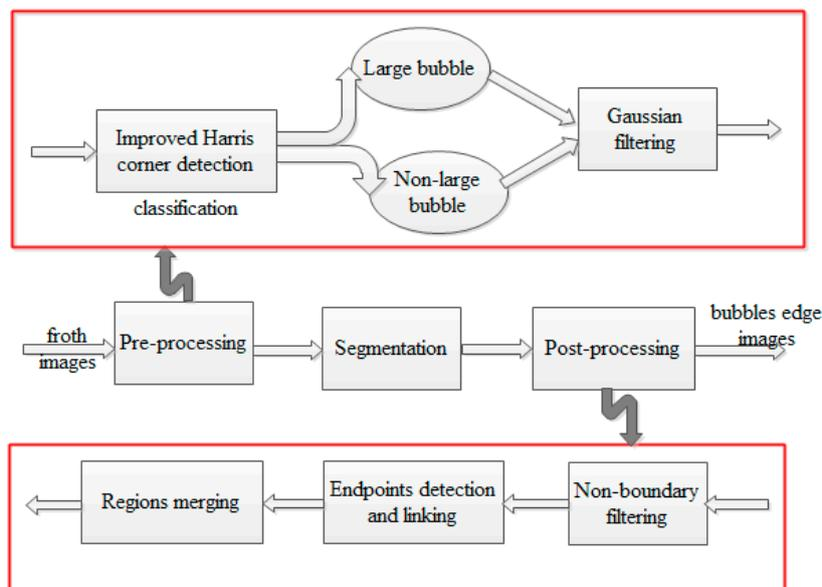
**Figure 11.** Working procedure of the proposed method.
