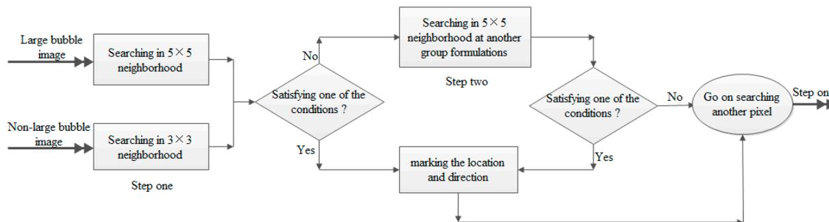
**Figure 5.** Algorithm workflow of the edge detection based on local gray value minima.
