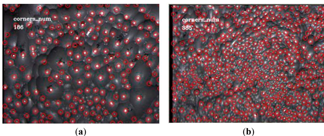
**Figure 8.** Improved Harris corner point detection. (a) Result of the large bubbles with tolerance distance 15; (b) Result of the small bubbles with tolerance distance 11.
