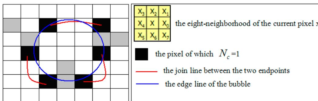
**Figure 10.** Gap linking diagram between the two endpoints and the representation of the pixels in the eight-neighborhood of the detecting pixel  $x$ .
