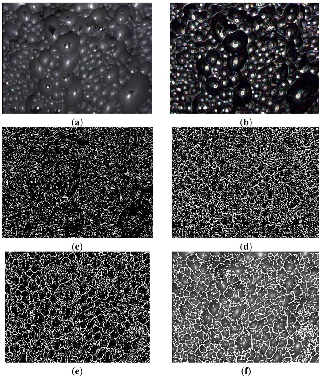
**Figure 12.** Comparison between the proposed edge detection algorithm and others (for the image of large bubbles). (a) Original image; (b) Sobel result; (c) Canny result; (d) Valley-edge result; (e) New algorithm result; (f) Result of overlap (e) and (a).
