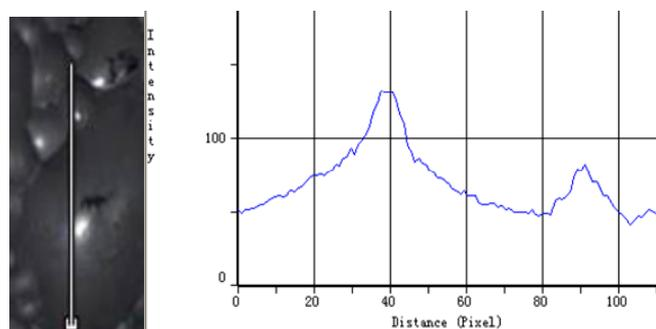
**Figure 3.** Gray value variation between two bubbles. **Left:** large bubble and the profile line; **Right:** the gray value histogram of the profile corresponding to the left image from bottom to top.
