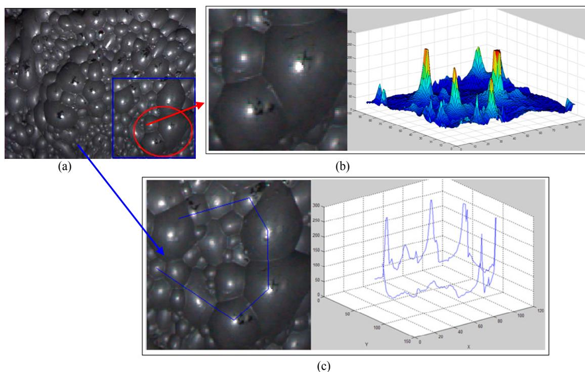
**Figure 1.** Gray value characteristics of the image of large bubbles. (a) a large bubble image; (b) left: a part of the image (a); right: the 3D surface of the left image; (c) left: large bubbles and the profile line; right: the gray level histogram of the profile corresponding to the left image.
