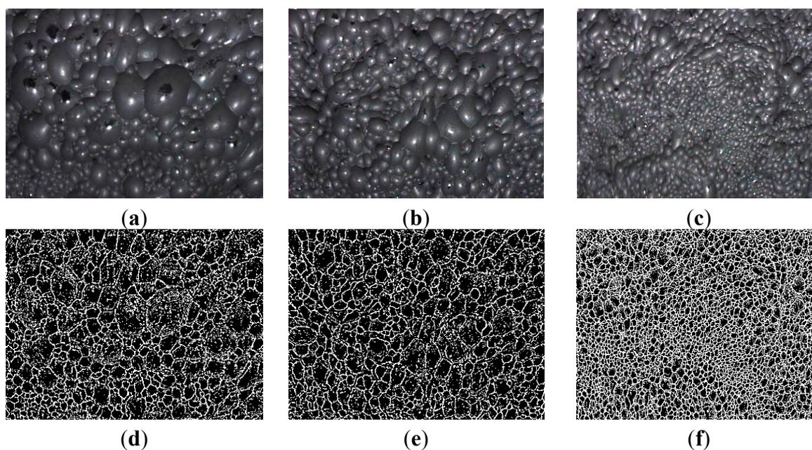
**Figure 6.** Edge detection results based on the proposed algorithm. (a–c) represent the original images of large, middle and small bubbles separately; (d–f) are the edge detection results corresponding to the images in (a), (b) and (c), respectively.
