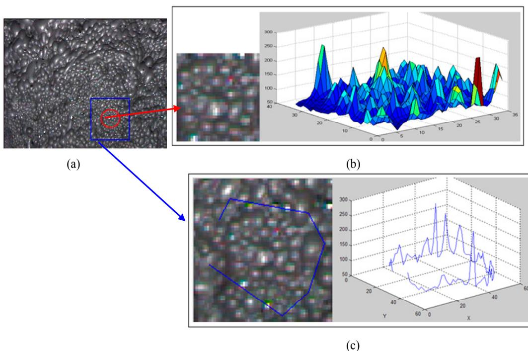
**Figure 2.** Gray value characteristic of the image of small bubbles. **(a)** A small bubble image; **(b) left:** a part of the image (a); **right:** the 3D surface of the left image; **(c) left:** small bubbles and the profile line; **right:** the gray level histogram of the profile corresponding to the left image.
