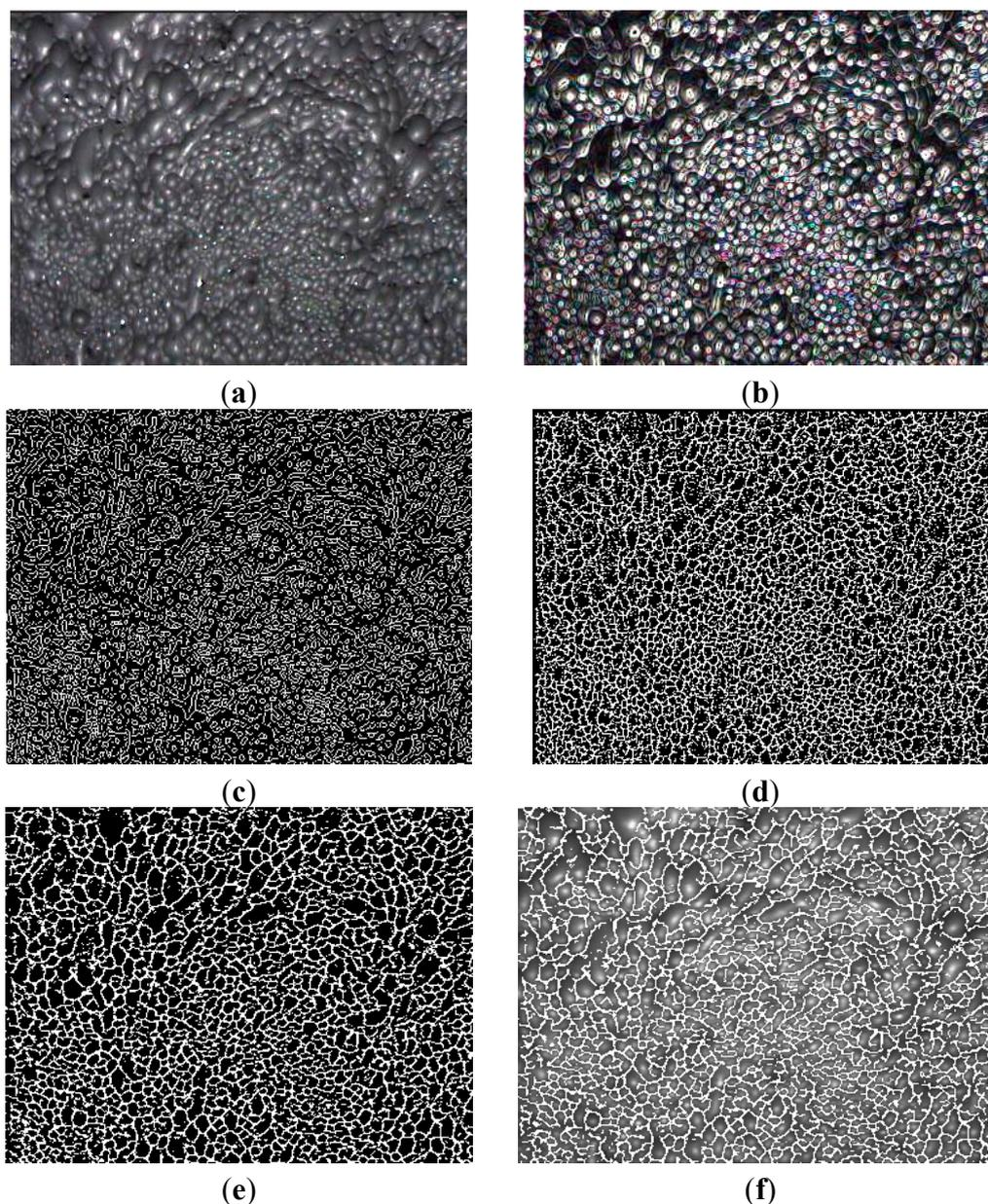
**Figure 13.** Comparison between the proposed edge detection algorithm and others (for the image of non-large bubbles). (a) Original image; (b) Sobel result; (c) Canny result; (d) Valley-edge result; (e) New algorithm result; (f) Result of overlap (e) and (a).
