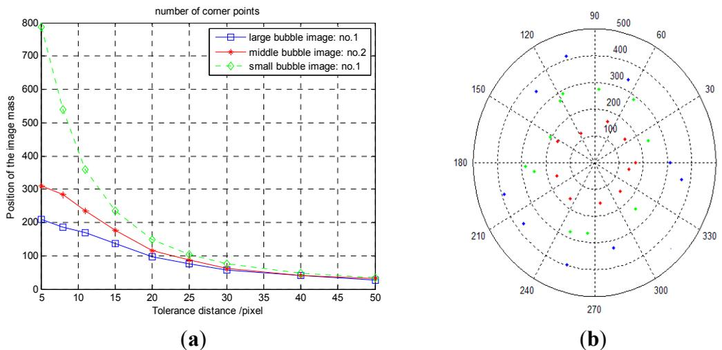
**Figure 9.** Corner point numbers (white spot numbers) distribution. (a) Corner point number distribution from Table 1; (b) Corner point number distribution of 30 different types of bubble images.
