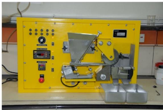
Figure 3.1: Lab-scale magnetic separator. (SGS.org, 2016)
