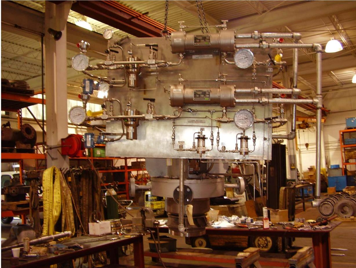
This mechanical sealing system requires virtually no maintenance and start up procedures are relatively simple, minimizing the potential for infant type failures.
