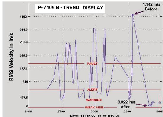
Figure 4. P-7109B Vibration Level before and after Installing the New Control System.
