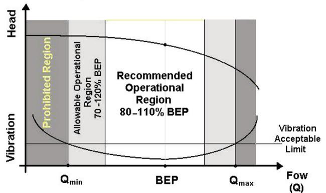
Figure 1. Pump Behavior × Operating Point.
