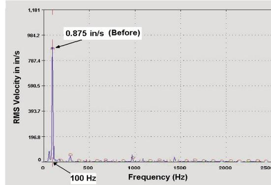
Figure 5. P-7109A—Frequency Spectrum at Nominal Speed: Dominant Vibration Peak of 0.875 in/s (22.23 mm/s), at ≈ 100 Hz (6000 cpm).
