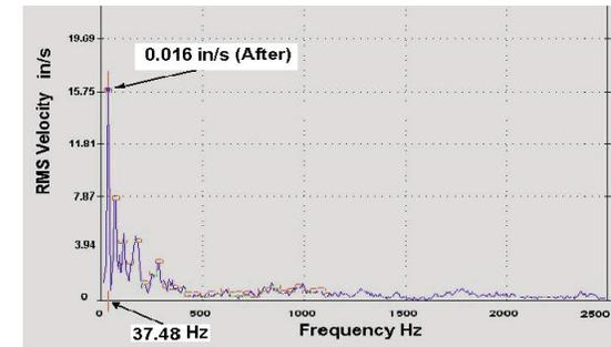
Figure 6. P-7109A—Frequency Spectrum after Dominant Peak of 0.016 in/s (0.4 mm/s, at Rotation Frequency 37.48 Hz (2249 cpm).
