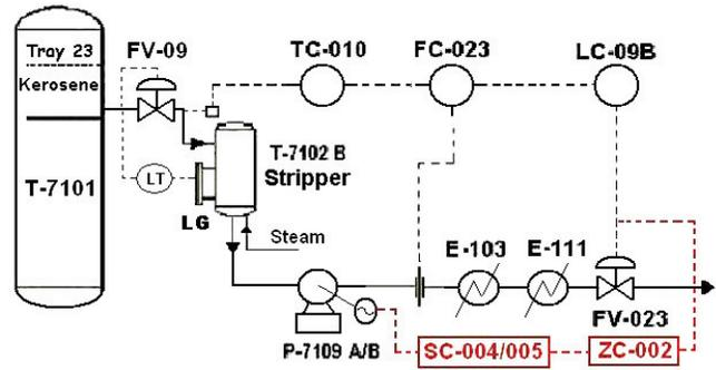
Figure 10. Simplified Flow Chart of P-7109 A/B System after Modification.
