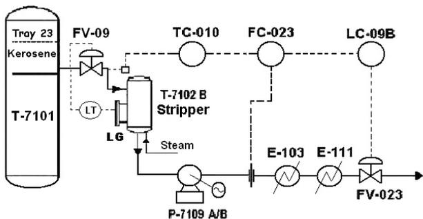
Figure 9. Simplified Flow Chart of P-7109 A/B System.
