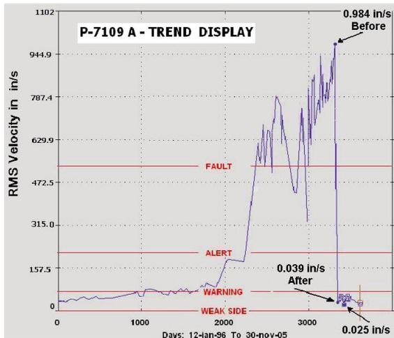
Figure 3. P-7109A Vibration Level before and after Installing the New Control System.
