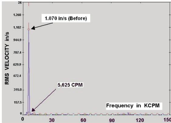
Figure 7. P-7109B—Frequency Spectrum at Nominal Speed: Dominant Vibration Peak of 1.07 in/s (27.19 mm/s) at 5625 cpm.
