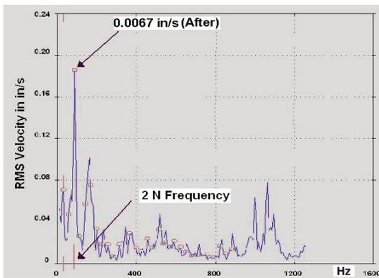
Figure 8. P-7109B—Frequency Spectrum after Dominant Peak of 0.0067 in/s (0.17 mm/s), at a frequency of  $2 \times N$ .
