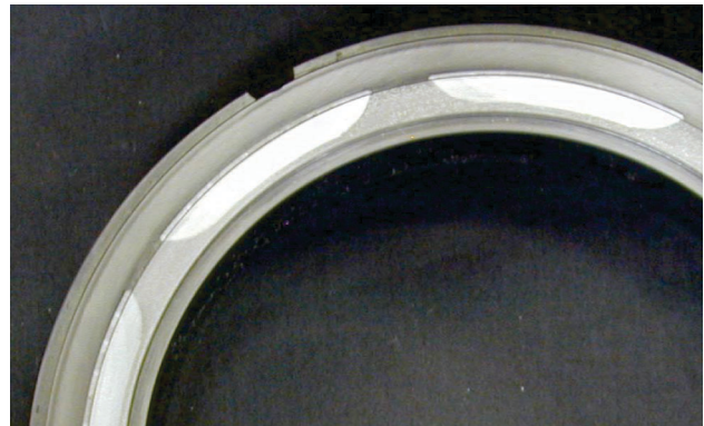
Figure 24. SiC Wavy after 4276 Field Hours.
