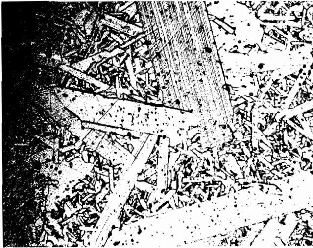
Figure 25. Optical Micrograph (400 ×) Showing Grain Growth in Sintered SiC.
