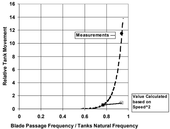
Figure 30. Relative Tank Movement Versus Blade Passage Frequency/Tanks Natural Frequency (300 kW Reactor, 12.5 m Diameter Tank) Data and Value based on Speed<sup>2</sup>.
