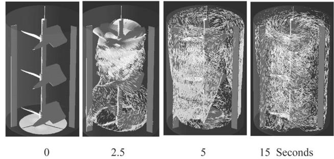
Figure 17. Hypertrace CFD Images of Three Up-Pumping A340 Impellers Versus Time.
