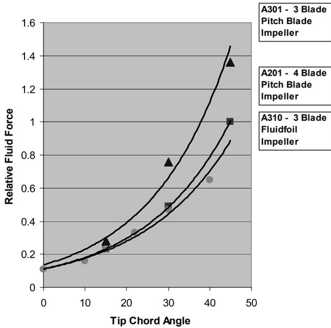
Figure 12. Relative Fluid Forces of A301, A201, and A310 Versus Tip Chord Angle.
