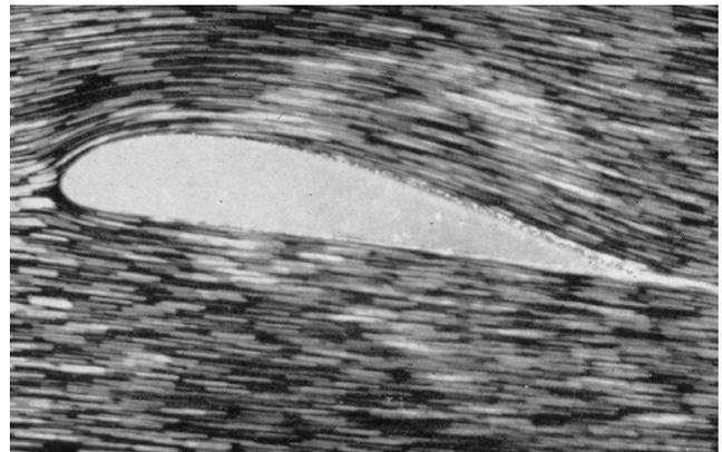
Figure 8. Streamlines Around an Airfoil Showing Nonseparated Flow.
