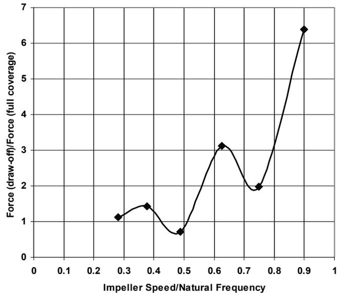
Figure 14. Force (Draw-Off)/Force (Full Coverage) Versus Impeller Speed/Natural Frequency (Three Bladed Impeller without Stabilizer).
