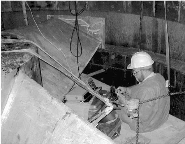
Figure 31. Setting up Instrumentation to Measure Fluid Forces on 210 inch Circulator Impeller.
