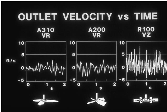
Figure 5. Outlet Velocity of Perpendicular Component Versus Time for A310, A200, and R100 Impellers.
