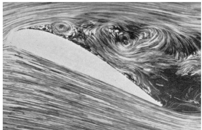
Figure 9. Streamlines Around an Airfoil Showing Separated Flow from a Higher Angle of Attack.
