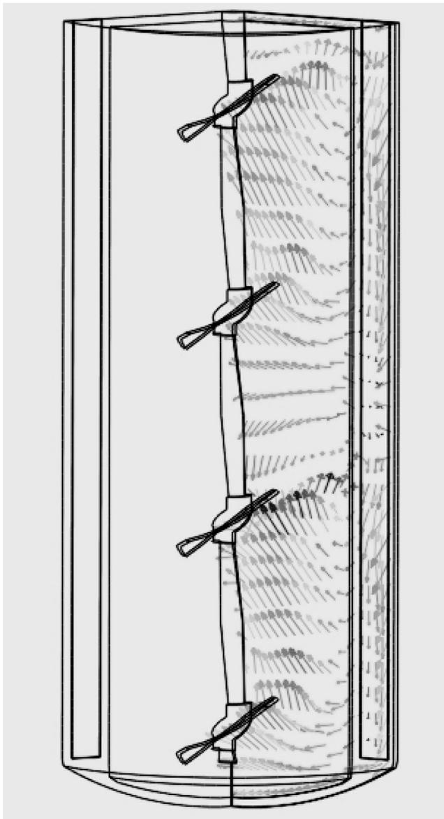
Figure 19. Velocity Vectors from CFD of Four A340 Up-Pumping Impellers.
