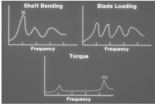
Figure 15. Frequency Spectrum of Shaft Bending, Blade Loading, and Torque.
