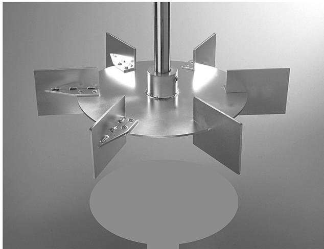
Figure 28. Impeller and Symmetric Sparge Configuration that Causes Excessive Axial Thrust.
