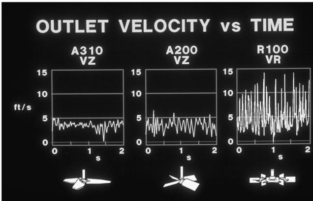
Figure 4. Outlet Velocity of Main Velocity Component Versus Time for A310, A200, and R100 Impellers.
