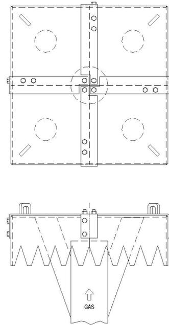
Figure 29. New Asymmetric Sparge Configuration that Reduces Axial Thrust.
