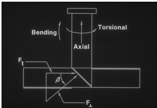
Figure 10. Fluid Forces (Bending, Torsional, and Axial) on a Mixing Shaft and Components on a Blade. Elevation View.
