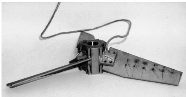
Figure 21. Strain Gauge Measurement of Impeller Hub.
