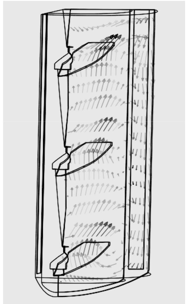
Figure 18. Velocity Vectors from CFD of Three A340 Up-Pumping Impellers.
