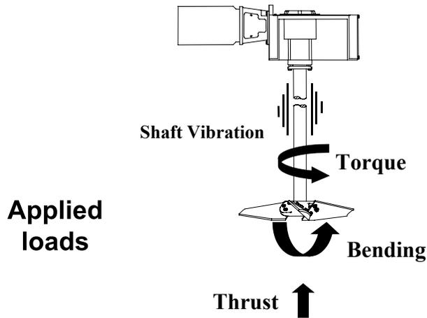
Figure 1. Fluid Forces Acting on a Mixer.
