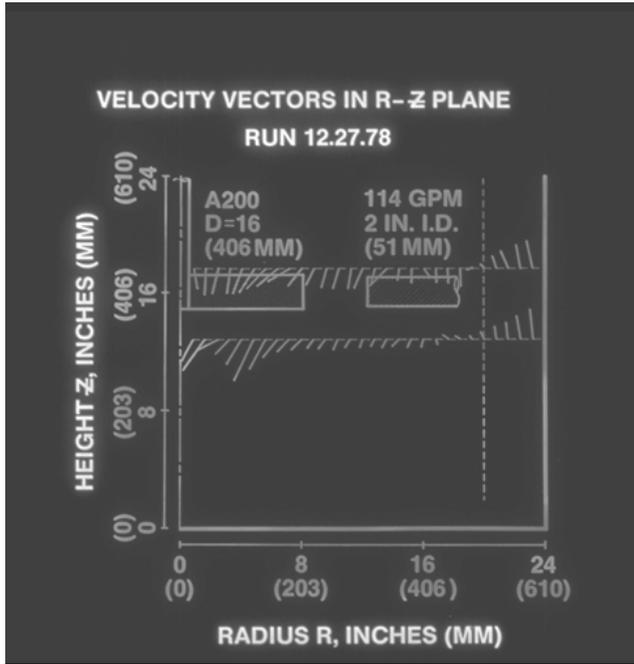
Figure 27. Velocity Vector Measurements of A200 Impeller with Inlet Side Flow at Impeller Location.
