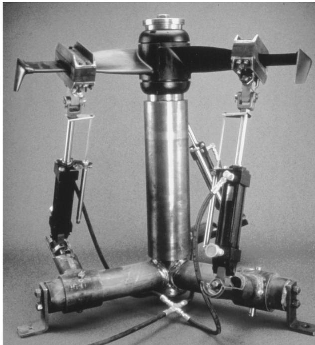
Figure 22. Fatigue Testing of Impeller Blades.
