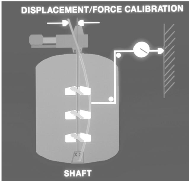
Figure 24. Calibration of Mixer for Fluid Forces.
