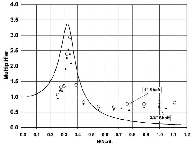
Figure 13. 15 Percent Damping Amplification Curve and 15.6 Inch A310 Impeller Fluid Force Measurements Versus Impeller Speed/Natural Frequency of Shaft.
