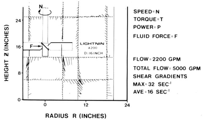
Figure 7. Velocity Vectors in the R-Z Plane for A200 Impeller. Also Showing Speed, Torque, Power, Horizontal Fluid Force, and Integrated Flow and Shear Gradients.
