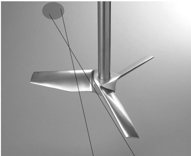
Figure 6. Laser Velocimeter Taking Velocity Measurements of a Mixing Impeller.
