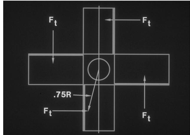
Figure 11. Resolving Torsional Loads on an Impeller to Show Blade Components. Plan View.
