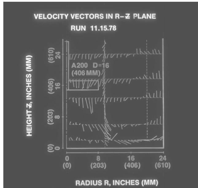
Figure 26. Velocity Vector Measurements of A200 Impeller.
