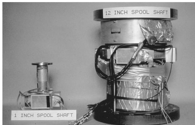
Figure 23. Shaft Spool Inserts for Measuring Fluid Forces on Lab Scale (1 Inch Diameter) and Full Scale (12 inch Diameter) Shaft.
