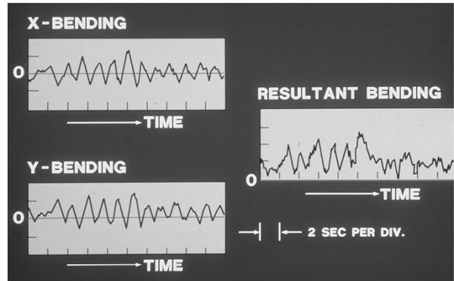
Figure 2. X-Bending, Y-Bending, and Resultant Bending on a Mixer Shaft.
