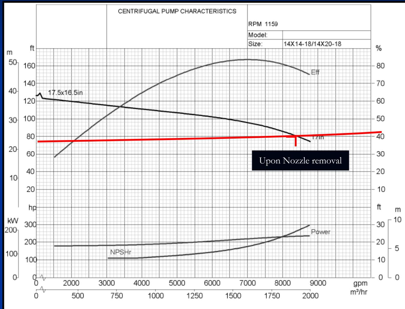
Flow = 8,400gpm    Head = 80 Ft.    NPSHr = 25Ft.    Hp = 232
