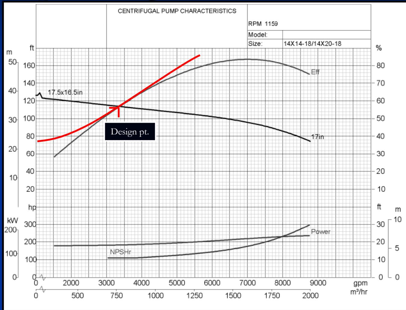
**Flow = 3,250gpm    Head = 112 Ft.    NPSHr = 11Ft.    Hp = 180**
