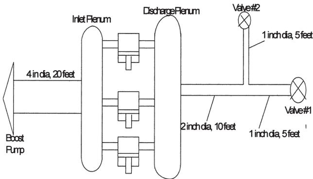
Figure 33. Schematic for Transient Simulation Example.
