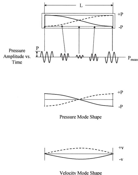
Figure 13. Pressure and Velocity Mode Shapes.
