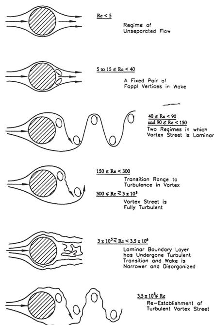
Figure 20. Vortex Streets. (Courtesy of Price and Smith, 1999, Turbomachinery Laboratory)
