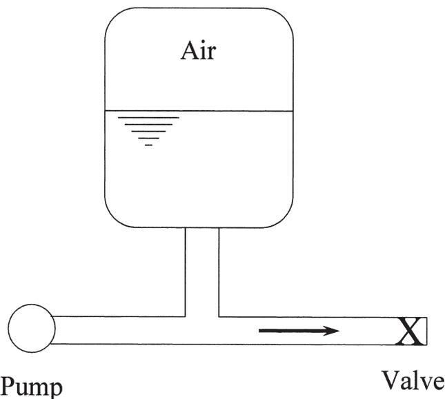
Figure 27. Use of Accumulator to Alleviate Water Hammer.
