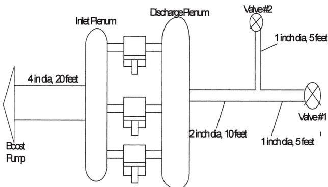
Figure 33. Schematic for Transient Simulation Example.
