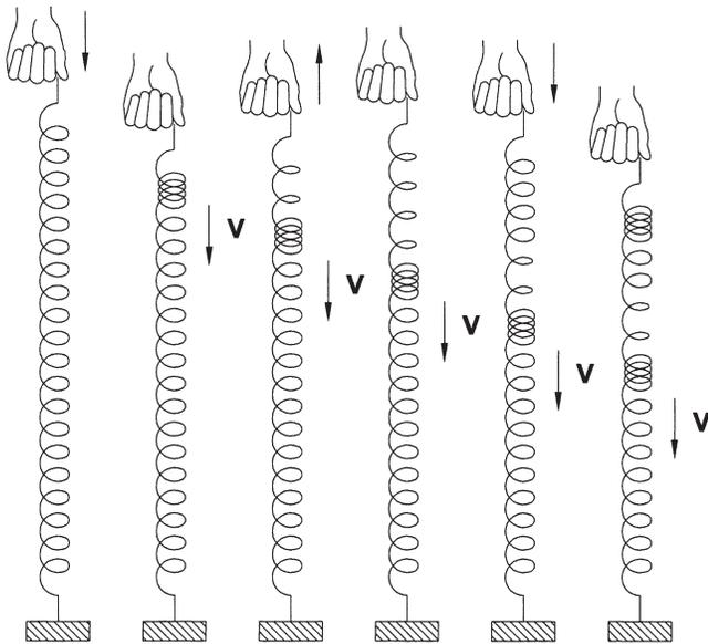
Figure 2. Example of a Longitudinal Wave.
