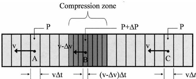
Figure 10. Close-Up View of Compression Wave.
