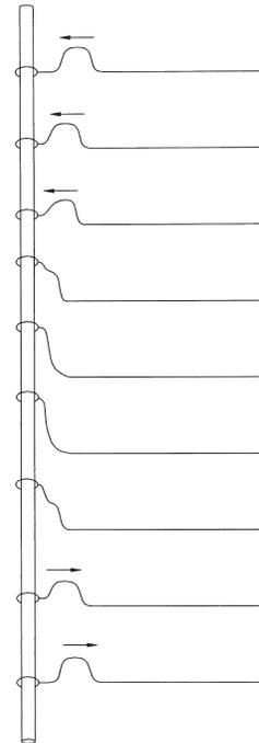
Figure 8. Reflection of a Vibrating String Pulse from a Free End.
