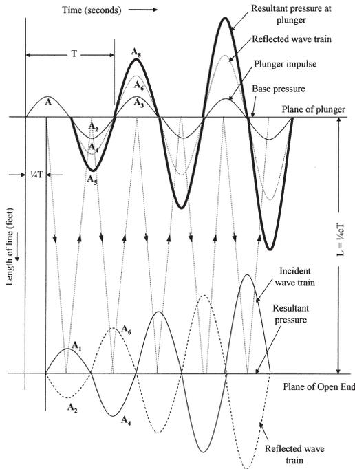
Figure 12. Illustration of Acoustic Resonance.
