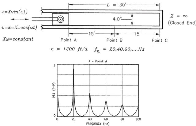
Figure 16. Typical Frequency Response. (Courtesy of Wachel and Tison, 1994, Turbomachinery Laboratory)
