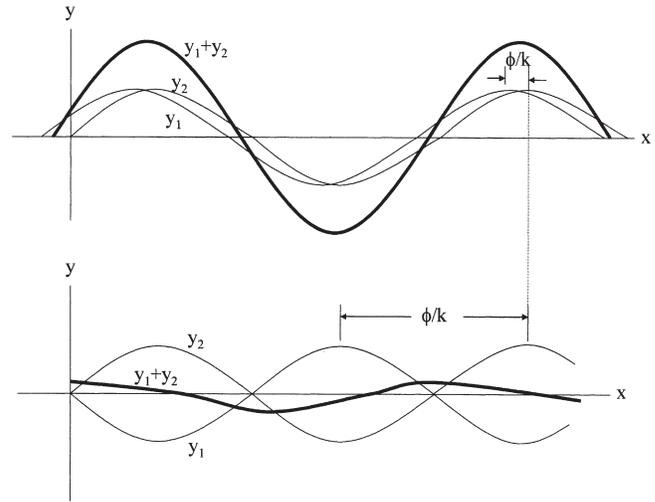
Figure 5. Constructive and Destructive Wave Interference.
