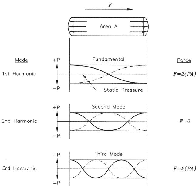
Figure 24. Shaking Forces Generated in a Vessel.
