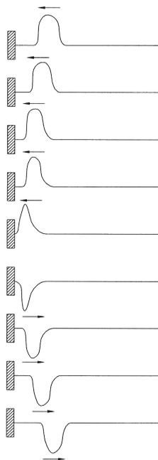
Figure 7. Reflection of a Vibrating String Pulse from a Fixed End.
