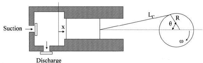
Figure 17. Schematic of Reciprocating Pump.
