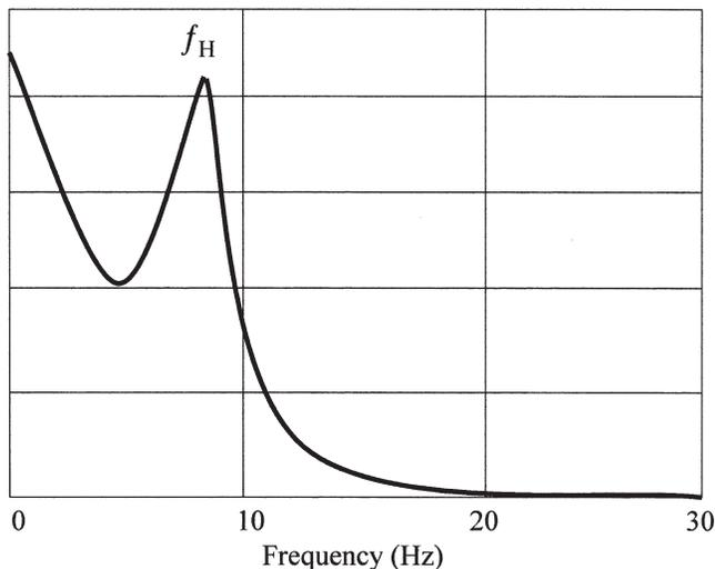
Figure 28. Typical Frequency Response of Volume-Choke-Volume Filter.
