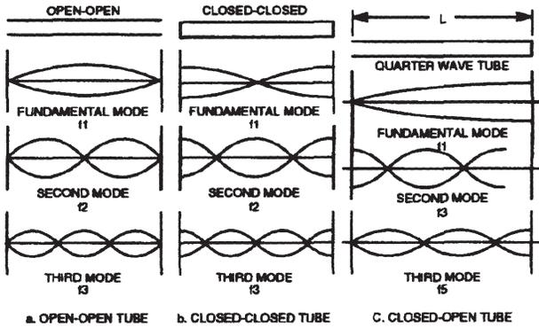
Figure 14. Pressure Modes Shapes for Organ Pipe Modes. (Courtesy of Jungbauer and Eckhardt, 1997, Turbomachinery Laboratory)
