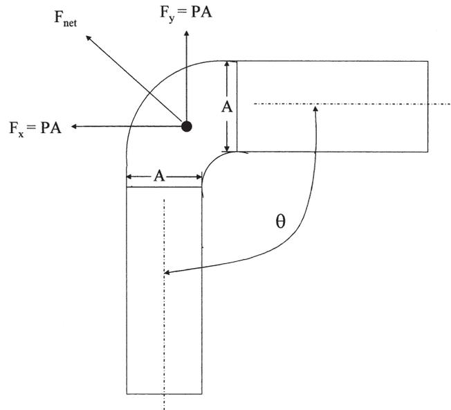
Figure 23. Shaking Forces Generated in an Elbow.
