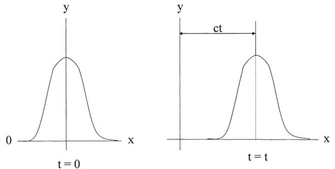
Figure 3. Pulse Traveling to the Right in a String.
