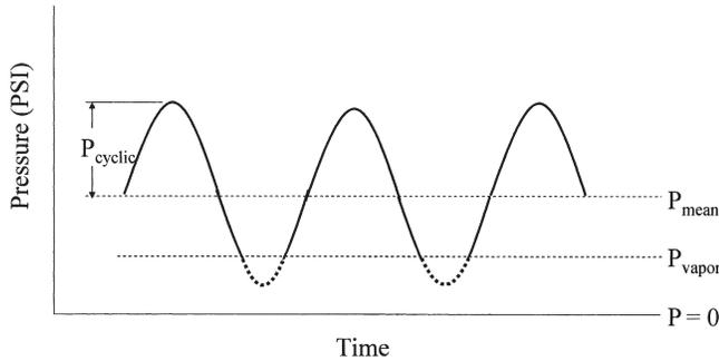
Figure 26. Pulsation-Generated Cavitation.
