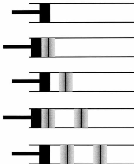
Figure 9. Generation of Acoustic Waves by a Piston.
