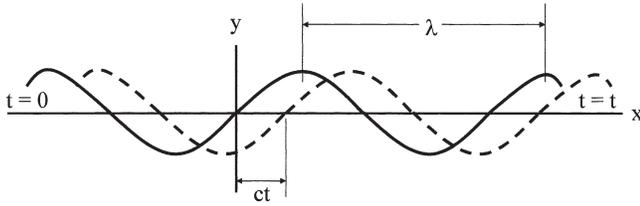
Figure 4. Sine Wave Traveling to the Right in a String.
