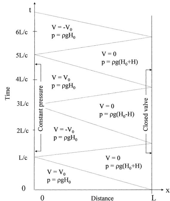
Figure 22. Illustration of Water Hammer in  $x$ - $t$  Plane.
