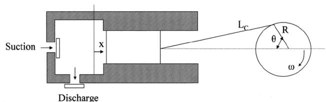
Figure 17. Schematic of Reciprocating Pump.
