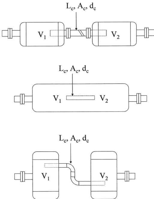
Figure 31. Possible Volume-Choke-Volume Filter Arrangements.
