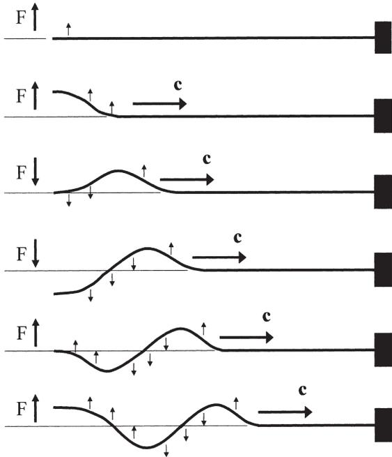
Figure 1. Example of a Transverse Wave.
