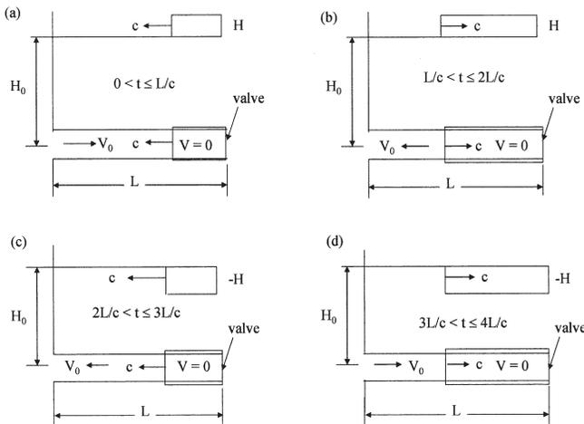
Figure 21. Illustration of Water Hammer.
