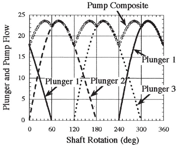
Figure 19. Triplex Pump Flow Excitations.
