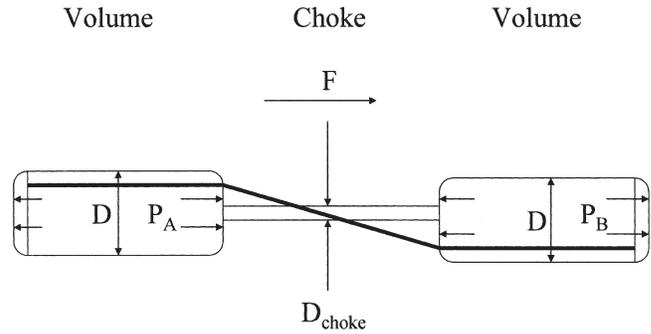
Figure 25. Shaking Forces Generated in Volume-Choke-Volume Filter.
