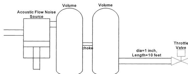
Figure 29. Schematic of Volume-Choke-Volume Simulation Case.
