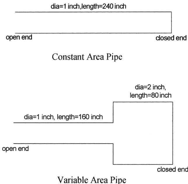
Figure 15. Constant and Variable Area Pipes.
