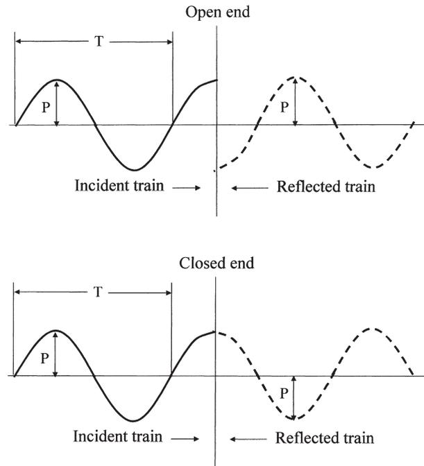
Figure 11. Reflection of Pressure Waves from Closed and Open Pipe Ends.
