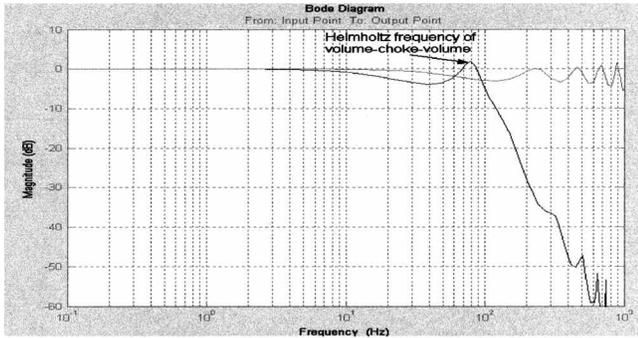
Figure 30. Volume-Choke-Volume Simulation Results.
