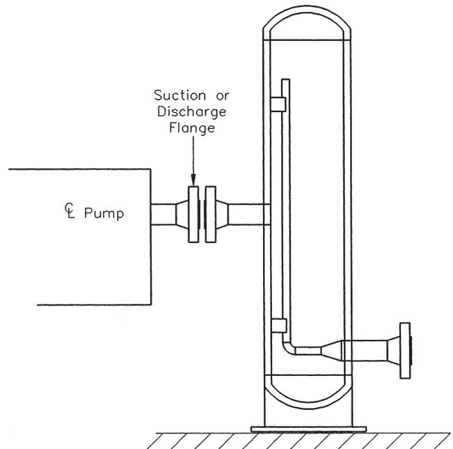
Figure 32. Volume-Choke All Liquid Filter. (Courtesy of Wachel and Tison, 1994, Turbomachinery Laboratory)
