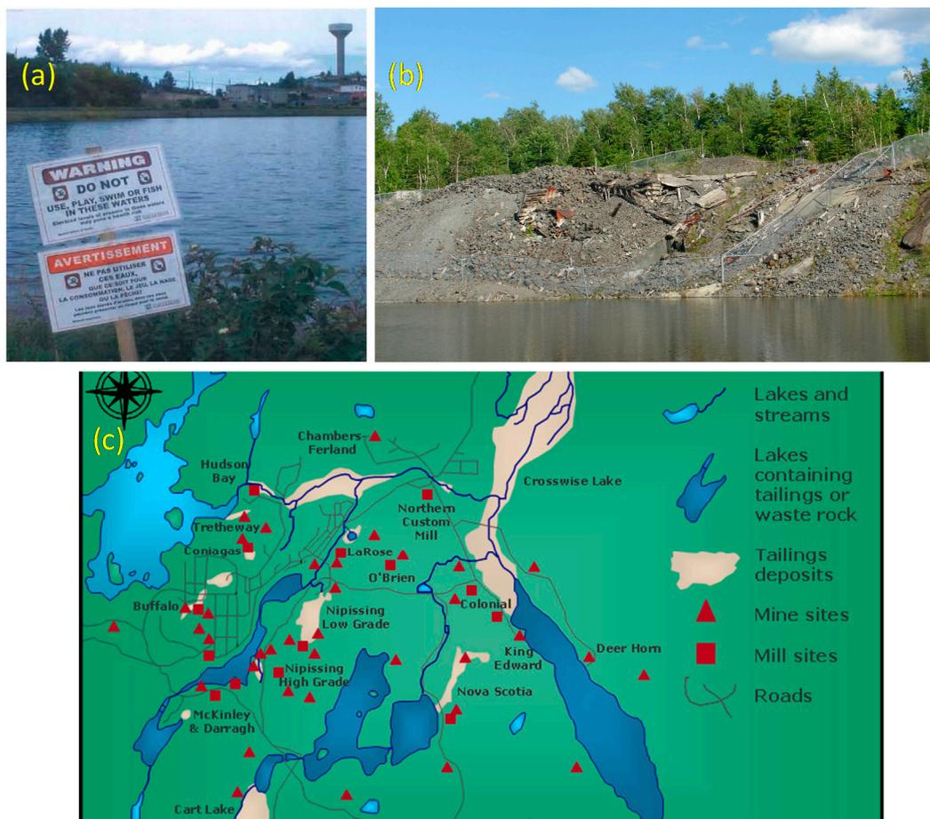
**Figure 8.** Water (a) and tailings (b) severely contaminated with arsenic; (c) Regional map of old workings in the region near Cobalt, Ontario, Canada with extensive tailings deposits indicated. Pictures from P.C. Miller, BacTech Environmental, reproduced with permission.
