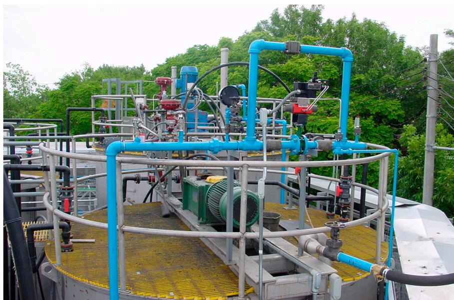
**Figure 5.** Bioleaching reactors at the Peñoles Mintek-Bactech demonstration plant at Monterrey, Mexico. Photograph by P.C. Miller, reproduced with permission.
