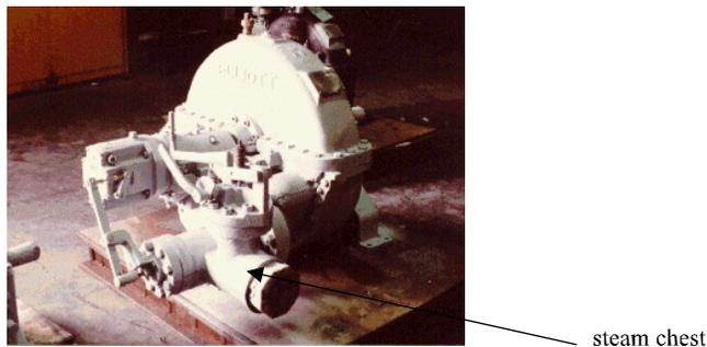
Figure 2. View from Inlet Side of Turbine.
