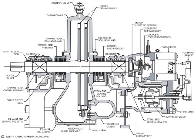
Figure 1. Cross Section of Typical Single-Stage Steam Turbine.
