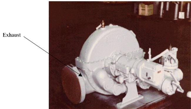
Figure 5. View from Exhaust End of Steam Turbine.
