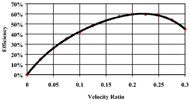
Figure 12. Typical Efficiency Curve for Single-Stage Turbine.
