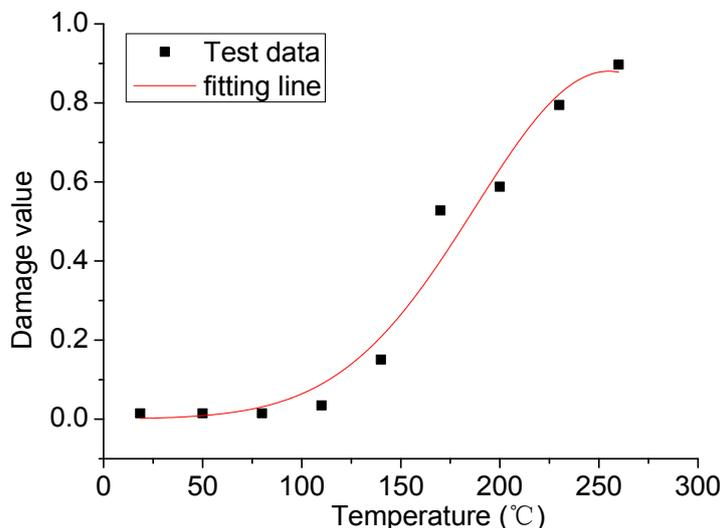
**Figure 7.** The relation between the temperature and damage.
