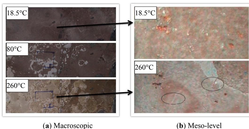
**Figure 3.** Thermal damage cracks of mudstone under high temperature.
