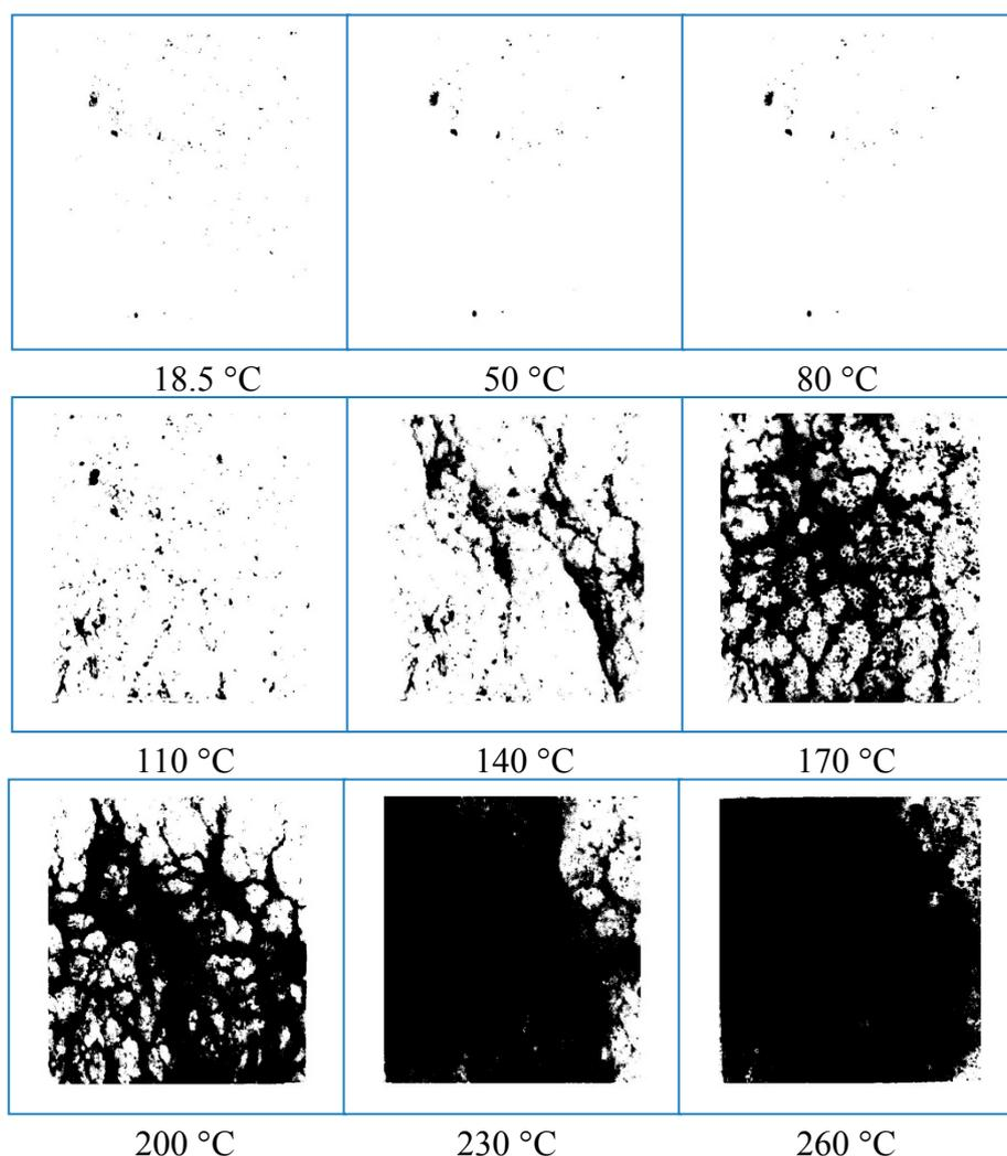
**Figure 6.** The grayscale and binary images of the rock salt surface thermal damage cracks at different temperature keep for 24 h from 18.5 to 260 °C.
