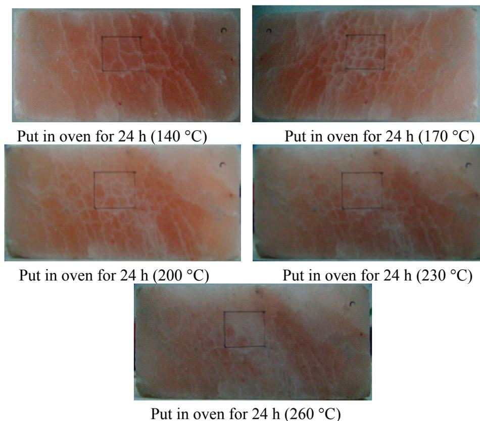
**Figure 5.** Comparison of the thermal damage cracks on the surface of rock salt in a given temperature region: 18.5, 50, 80, 110, 140, 170, 200, 230 and 260 °C.
