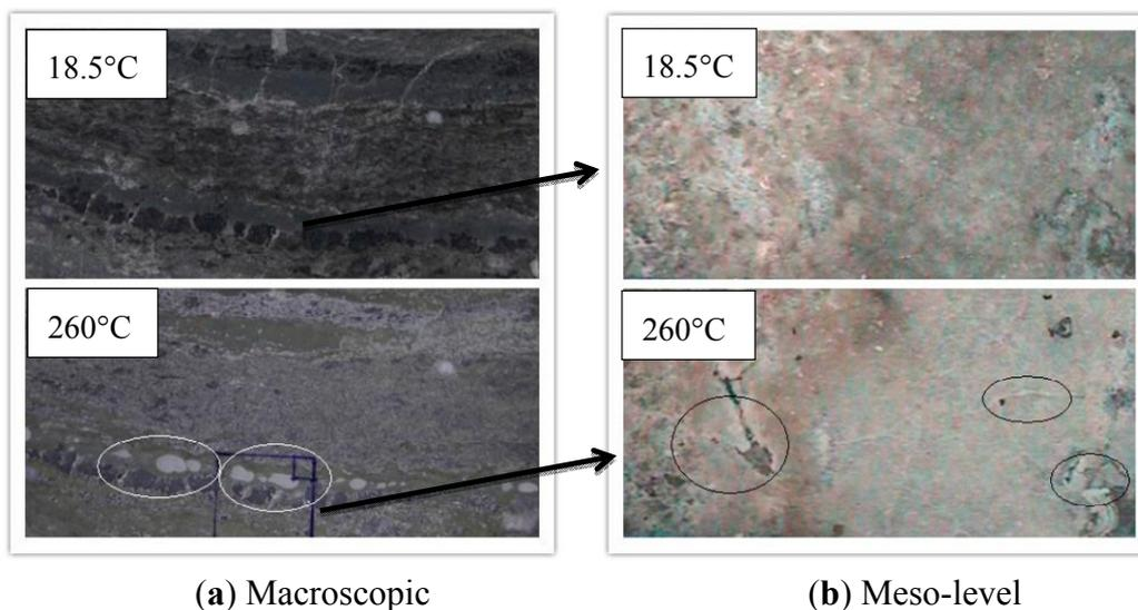
**Figure 4.** Thermal damage cracks of gypsum under high temperature.
