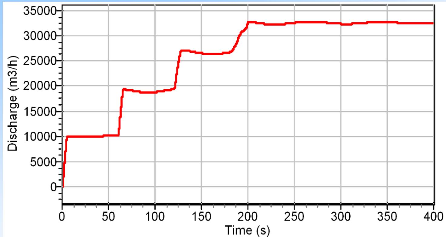
Cooling water flow through condenser at start-up
