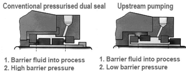
Figure 1. Simplified Scheme of Upstream Pumping Versus Conventional Double Pressurized Seal Working Principle.
