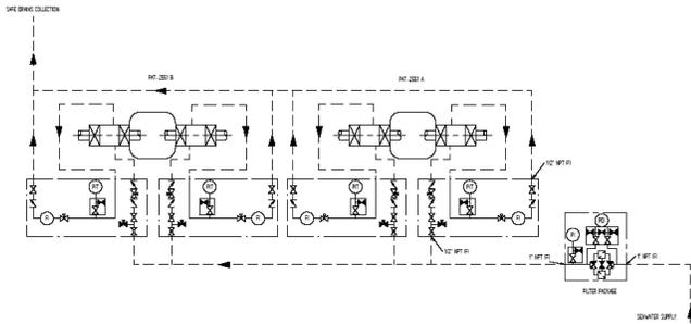
Figure 4. Filtered Sea Water Flow Diagram.
