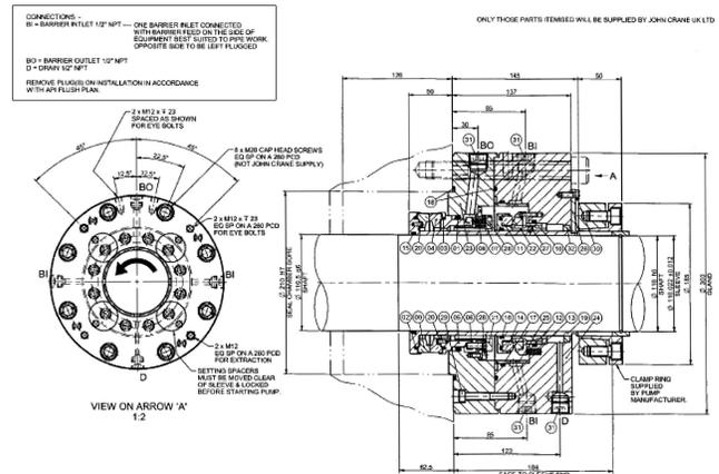
Figure 3. Upstream Pumping Seal.
