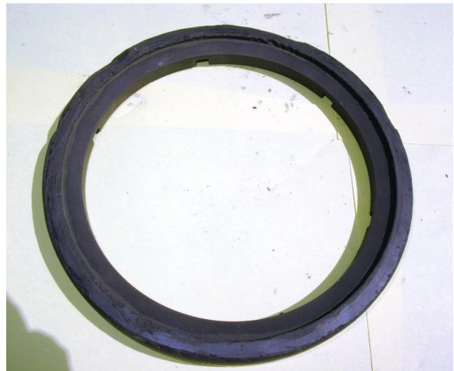
Figure 5. Damaged Inboard Primary Ring.
