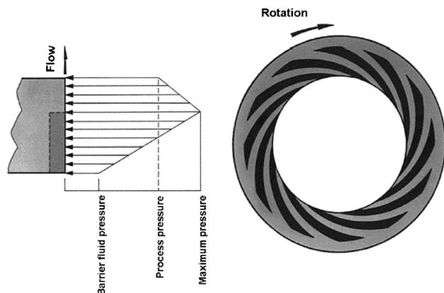
Figure 2. Spiral Grooved Mating Ring.
