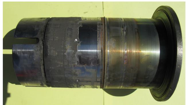
Figure 6. Damaged Shaft Sleeve.
