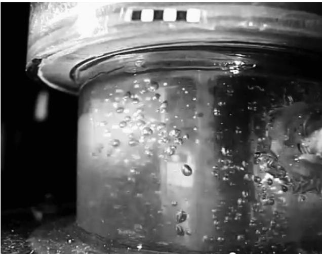
Figure 24. Gas Pocket (Regimes II and III, Point (4), Figure 16) at Intake.
