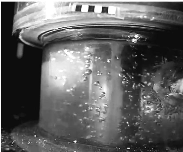
Figure 20. Bubble Flow (Regime I, Point (2), Figure 16) at Intake.
