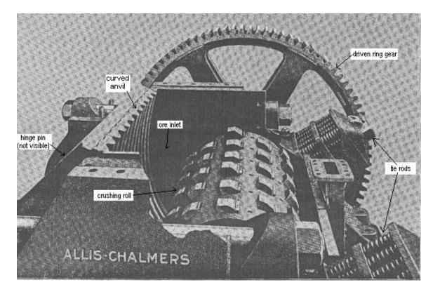
This monster piece of equipment is an engineering wonder. Such crushers continued to be promoted in the trade into at least the `50's even though their capacity was limited. The industry doesn't expect more than a 2:1 reduction (for example, 8" thick rocks would be crushed to 4") from single roll crushers. Much higher reductions can be had with the coffee grinder and hammer style crushers.
