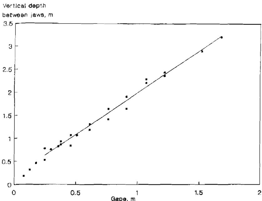
Fig. 2 — Variation of vertical depth between jaws with gape for jaw crushers.
