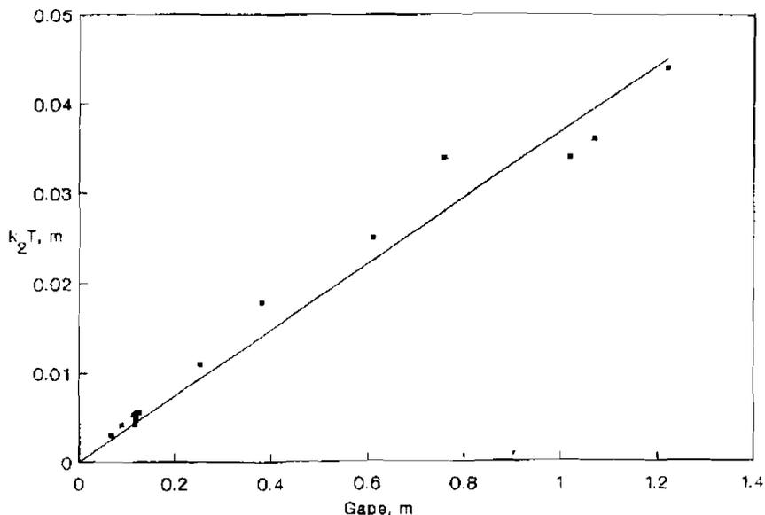
Fig. 3 — Variation of  $K_2T$  with gape for jaw crushers.
