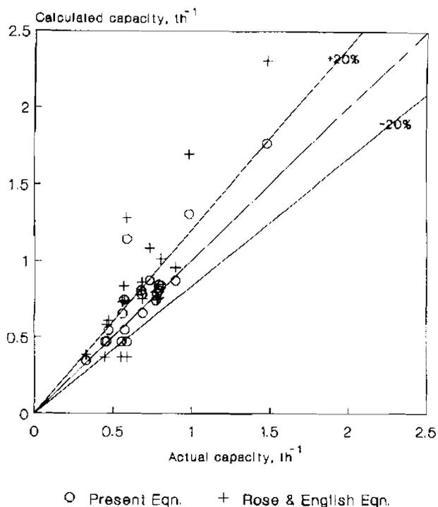
Fig. 1 — Comparison of calculated capacities with the data of Hersam (1923) for different machine parameters.
