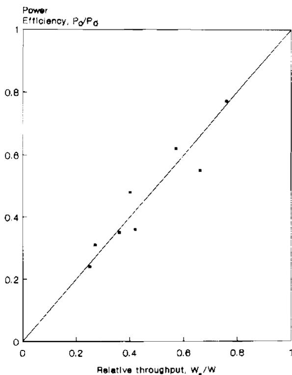
Fig. 4 — Relation between power efficiency and relative throughput for jaw crushers
