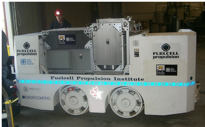
Figure 1–Fuel cell-powered mine locomotive of Vehicle Projects Inc. Utilizing PEM fuel cells and reversible metal-hydride storage, this pure fuel cell vehicle was successfully demonstrated in a working underground gold mine in 2002
