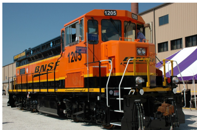
Figure 2-Hydrogen fuel-cell hybrid switch locomotive developed by Vehicle Projects Inc. The 130 t locomotive, developed in partnership with BNSF Railway, completed its successful demonstration at a rail yard in Los Angeles, California, in 2010
