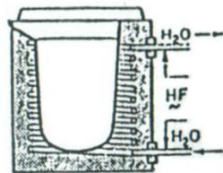
Coreless type high frequency induction melting furnace
