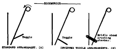
**Fig. 5—Standard and inverted toggle arrangements in single-toggle crushers.**
