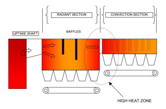
Figure 19: Planned waste heat boiler baffle installation
