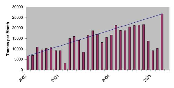
Figure 11: Improvement in Steam Dryer throughput
