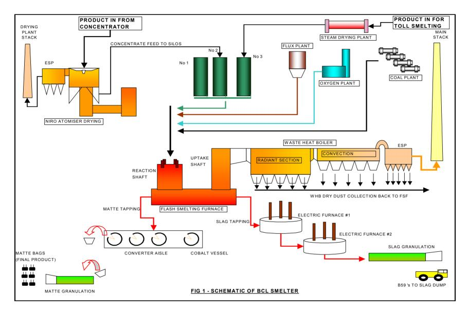
Figure 1: BCL Smelter Plant Flowsheet
