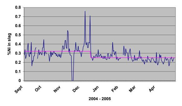
Figure 14: Nickel content of discard slag
