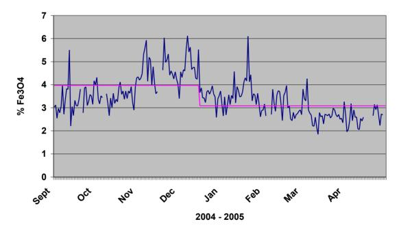
Figure 13: Magnetite levels in discard slag
