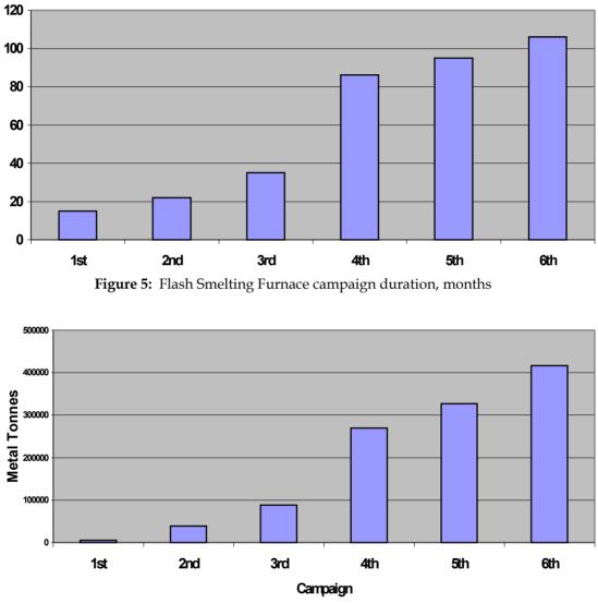
Figures 6: Flash Smelting Furnace metal production per campaign
