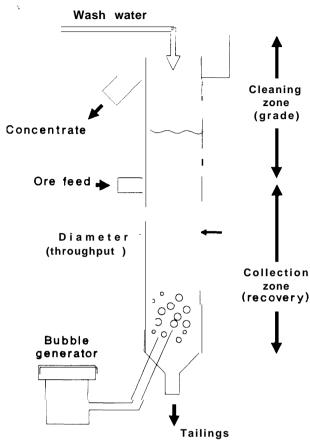
Column cells already are used for molybdenum concentration, and are being tested in copper milling. Experience with a column cell at San Manuel, Arizona showed a concentrate grade of 29.83 percent copper with a sulfide copper recovery of 90.36 percent, compared to the conventional San Manuel flotation circuit with 29.99 percent copper in the concentrate and a recovery of 90.12 percent .51
