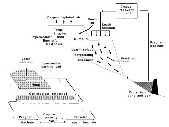
Figure 6-13.-Heap and Dump Leaching
