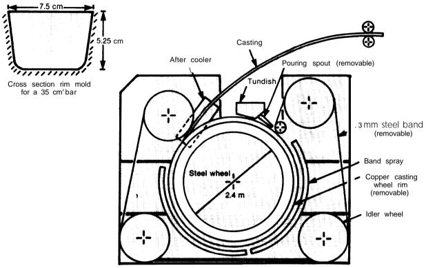
Figure 6-30.—Continuous Casting Wheel
