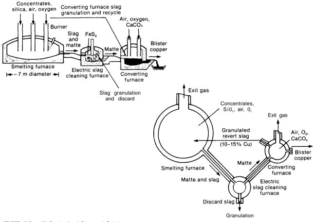
Figure 6-27.— Mitsubishi Continuous Smelting System
