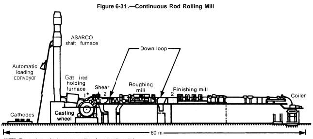
\*NOTE The numbers refer to sensor positions for automatic control
