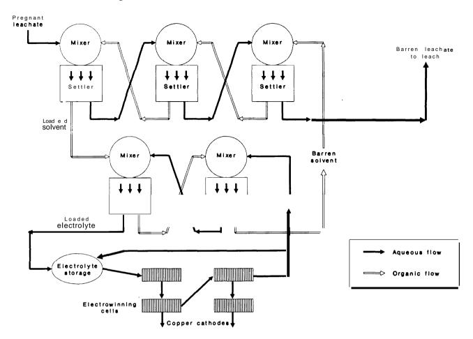
Figure 6-29.-Flowsheet for Solvent Extraction
