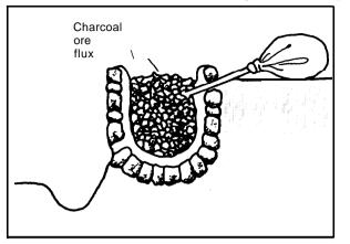
The Egyptian copper smelting furnace was filled with a mixture of copper ore, charcoal and iron ore to act as a flux. It was blown for several hours by foot or hand bellows.
