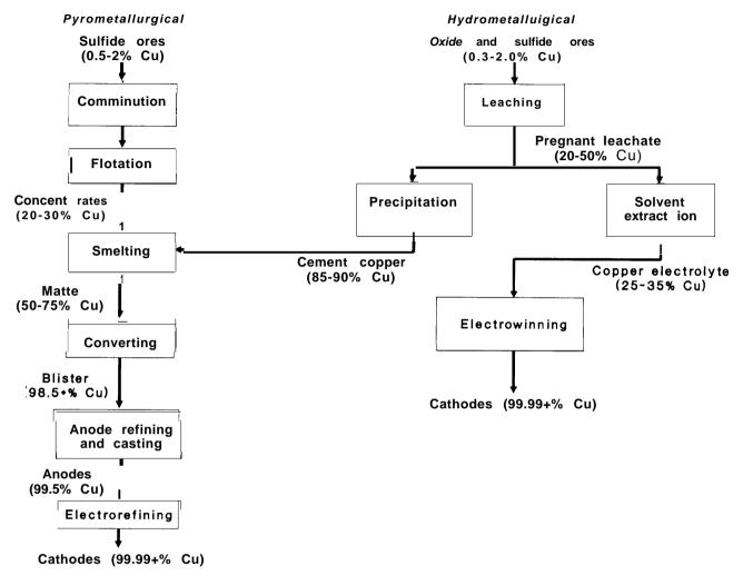
Figure 6-1.-Flow Sheets for Copper Production
