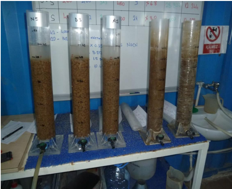
Figure 4: QC pellet testing at a gold heap leach operation
