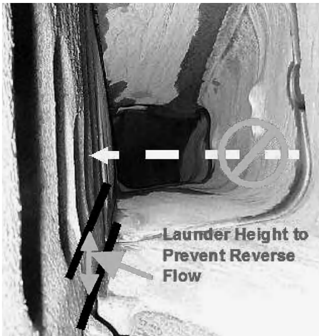
Figure 13 — Control of “static” reverse flow.
