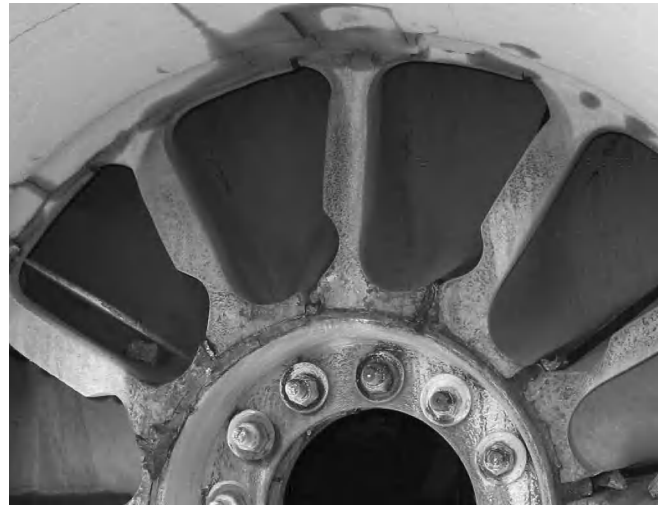
Figure 19 — Trunnion-side discharge cone — curved pulp lifter (after Dunn et al., 2006).
