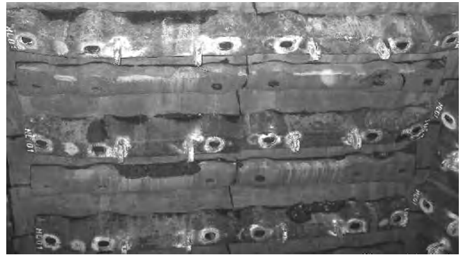
Figure 3 — Traditional “HiLo” plate and lifter shell lining (after Dunn et al., 2006).
