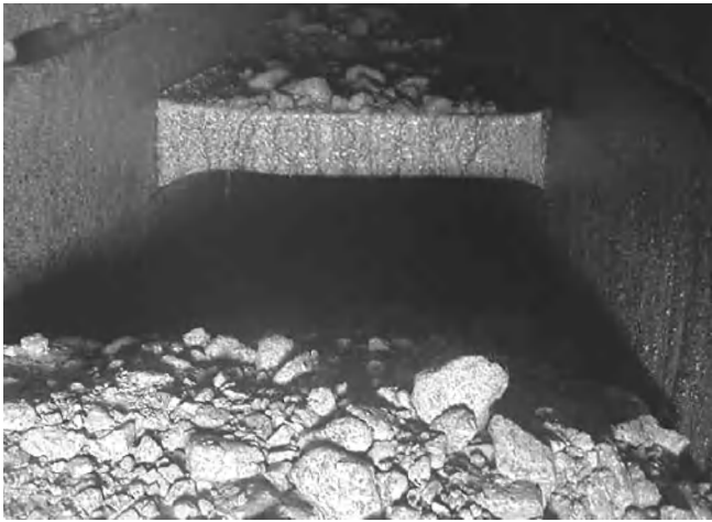
Figure 10 — Rocks in pulp-lifter channel following a crash stop (after Hart et al., 2001).
