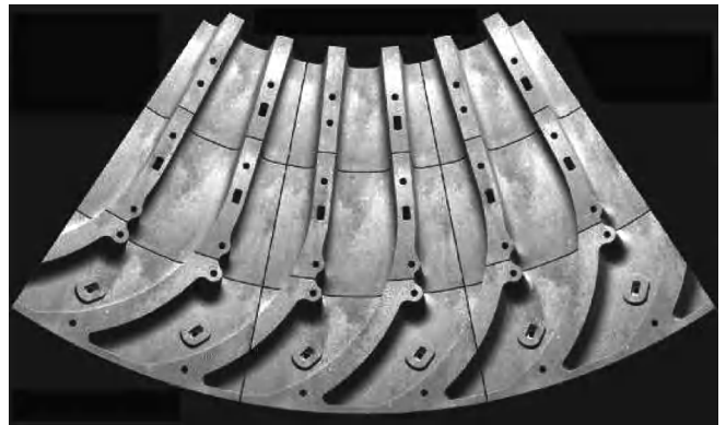
Figure 16— Illustration of an array of “hockey-stick” curved pulp lifters.
