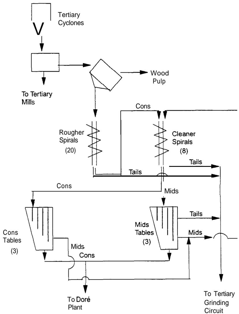
FIG 5 - Gravity plant flowsheet.
