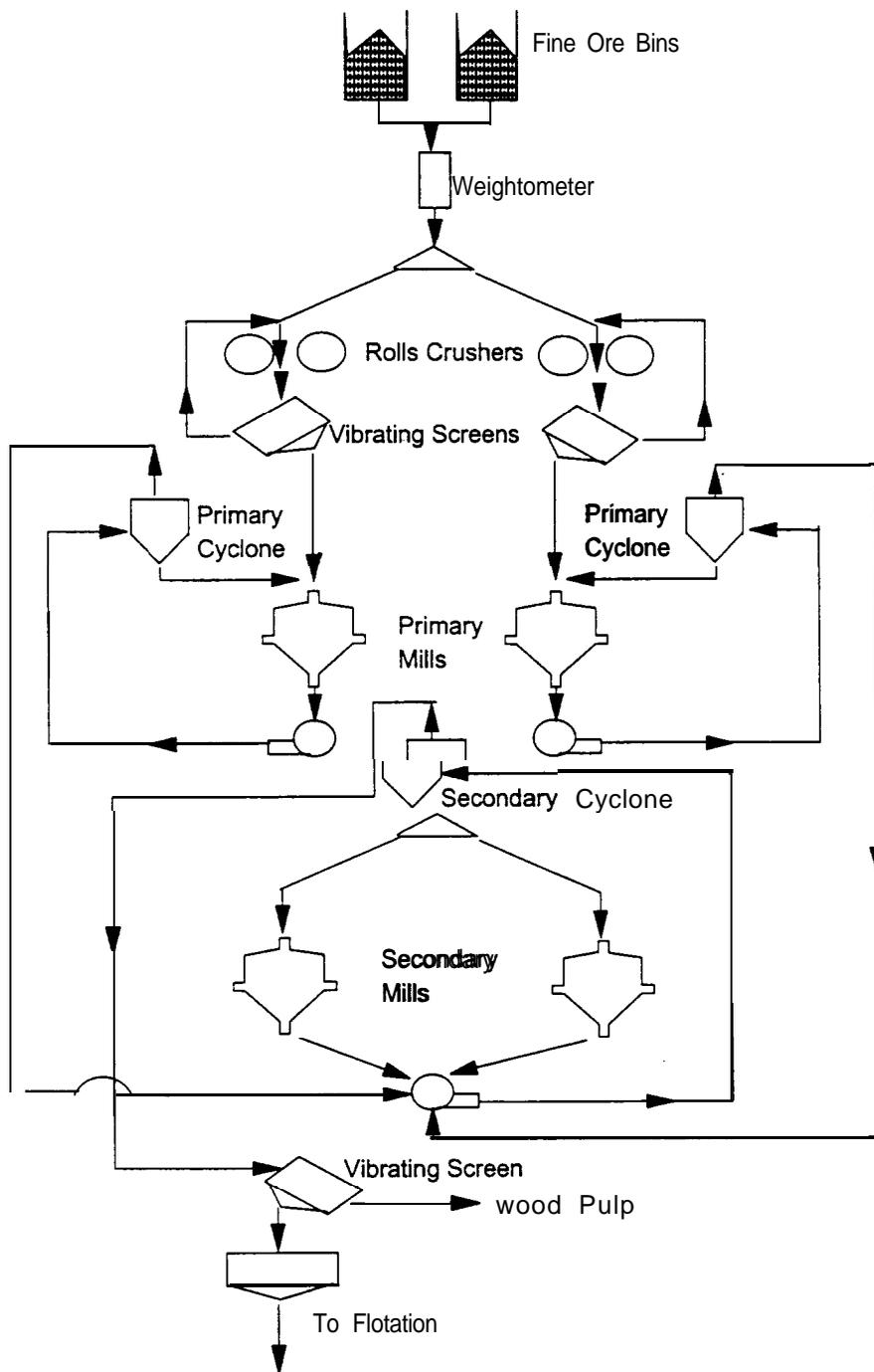
FIG 1 - Grinding circuit flowsheet.
