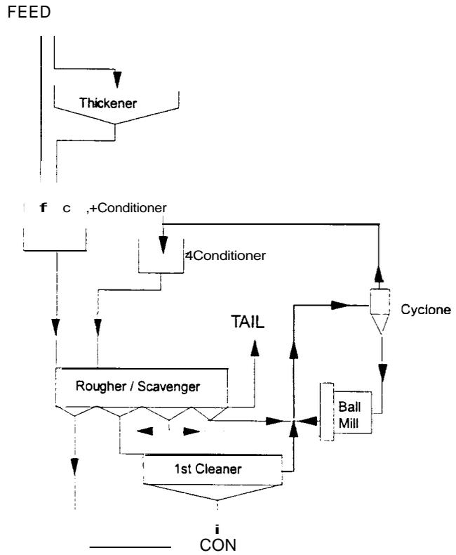
FIG 4 - Zinc flotation circuit.
