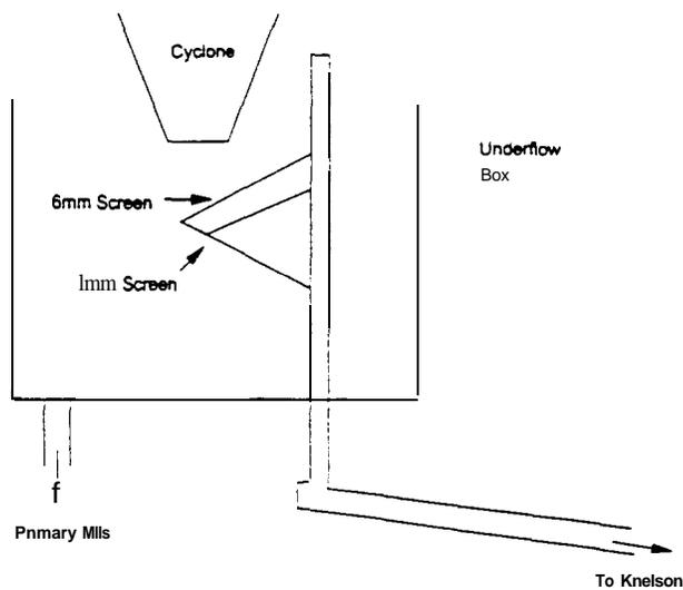
FIG 8 · Cyclone underflow screen / cutter.
