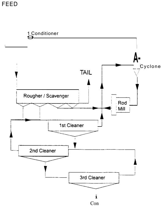
FIG 3 - Lead flotation circuit.
