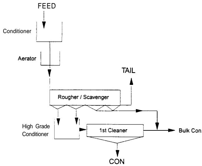
FIG 2 - Copper flotation circuit
