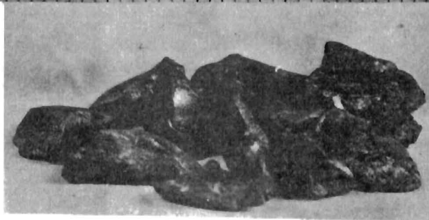
Figure 1.-- Original minus 2 plus 3 mesh bornite before leaching
