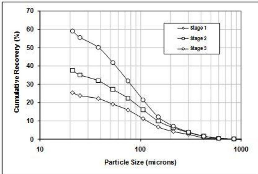
Cumulative GRG Recovery as a Function of Particle Size
