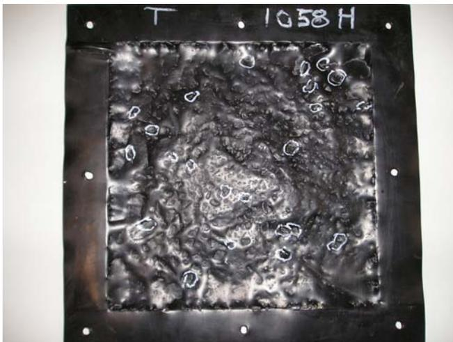
Photo 3: 1.5mm HDPE tested for puncture at 60°C
