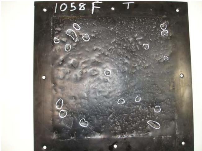
Photo 2: 1.5mm HDPE tested for puncture at 21°C.
