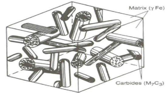
Schematic showing the heterogeneous micro-structure of high-chromium white irons.
