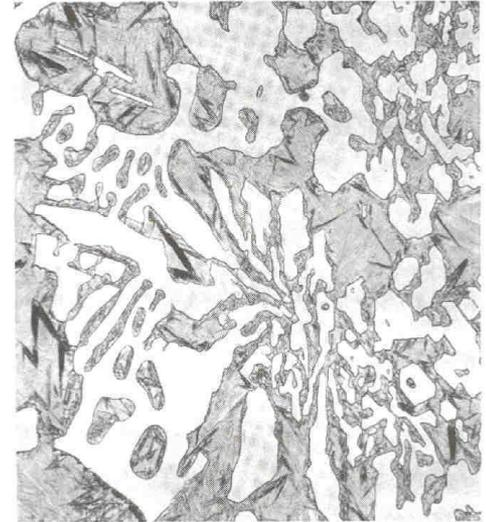
Typical microstructure of class I type D nickel-chromium white cast iron.
