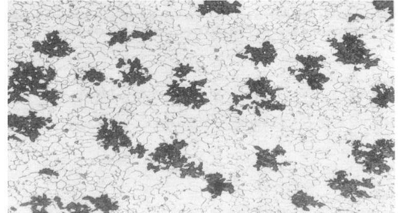
Microstructure of Malleable Iron
