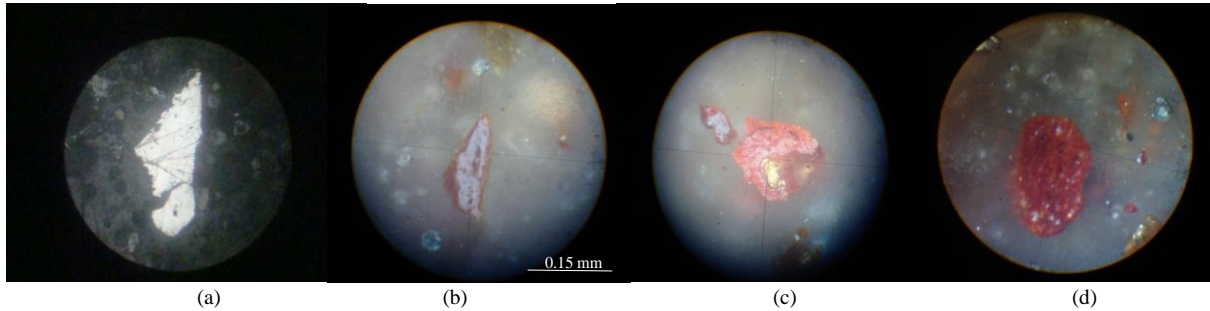
Figure 3. Photomicrographs showing the conversion of pyrite to hematite during roasting (a) pyrite particle in the concentrate (b) partially oxidized pyrite with a boundary of hematite (reddish) after 5 min roasting (c) pyrite in an advanced stage of conversion to hematite after roasting for 10 min (d) hematite produced after 20 min
