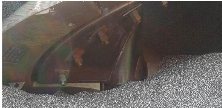
Figure 18 – View inside the Vertimill after the media charge unloading
