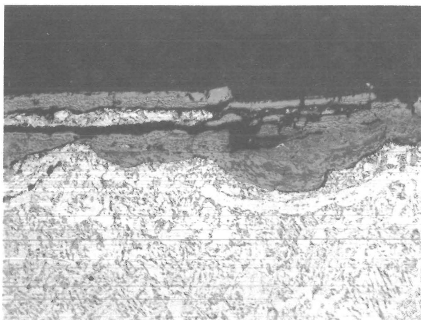
FIGURE 5. - Flaking of surface of steel ball (X 200) subjected to repeated impacts. Ball from alloy 1 after 530,000 impacts. Dark gray in upper region is plastic mounting material, gray near middle is oxidized iron, lower region is martensitic steel.
